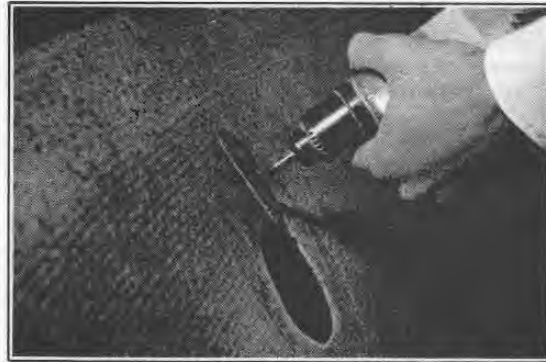
Figure 2-81. Rough Sanding Inside Surface
