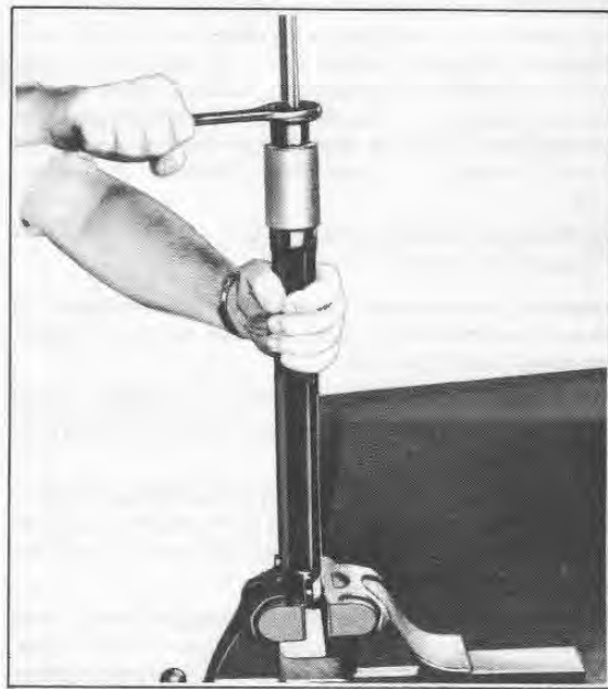
Figure 2-43. Removing Fork Slider Bushing
