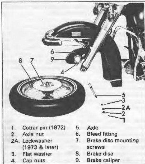
Figure 2-6. Front Wheel - FL (1972 and Later)
