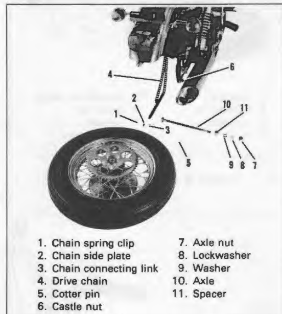
Figure 2-12. Removing Rear Wheel (1973 and Later)
