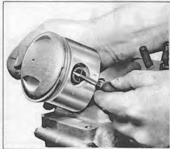
Figure 3-9. Removing Piston Pin Lock Ring (1972 and Earlier)
