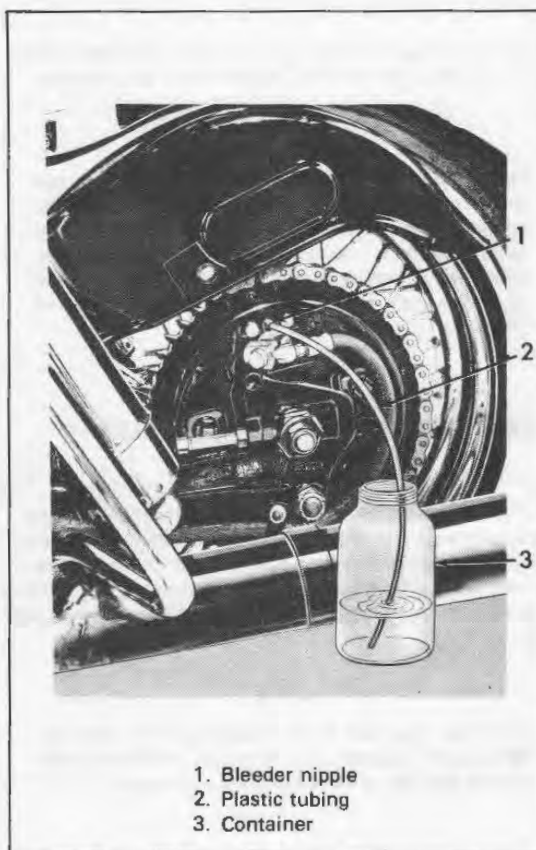
Figure 2-69. Bleeding Hydraulic Brake System
