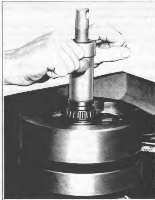
Figure 3-49. Pressing Bearing on Sprocket Shaft
