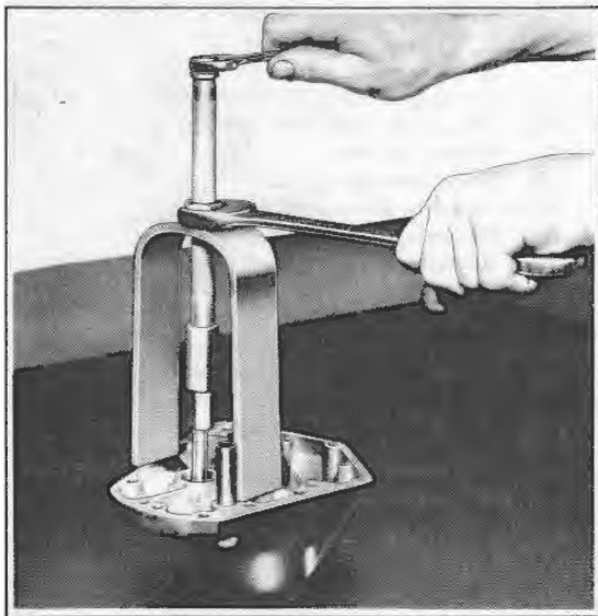
Figure 3-31. Removing Pinion Shaft Cover Bushing
