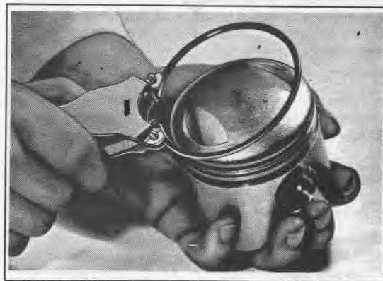
Figure 3-15. Assembling Rings with Ring Expander
