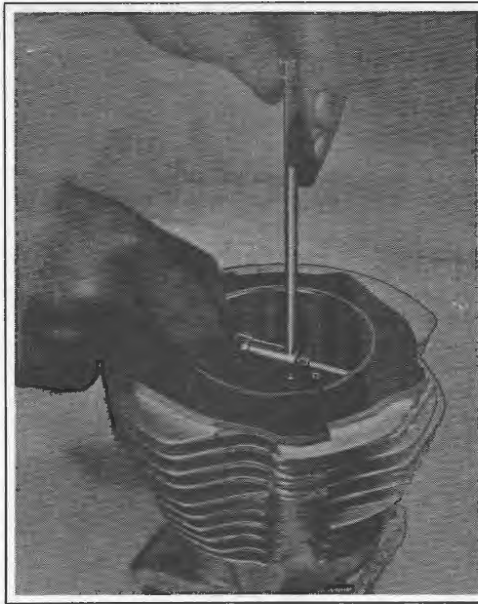
Figure 3-11. Measuring Cylinder Bore
