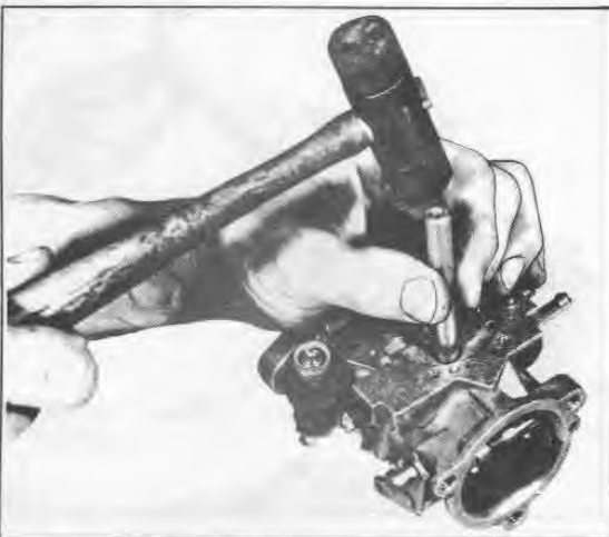
Figure 3-62. Removing Main Nozzle
