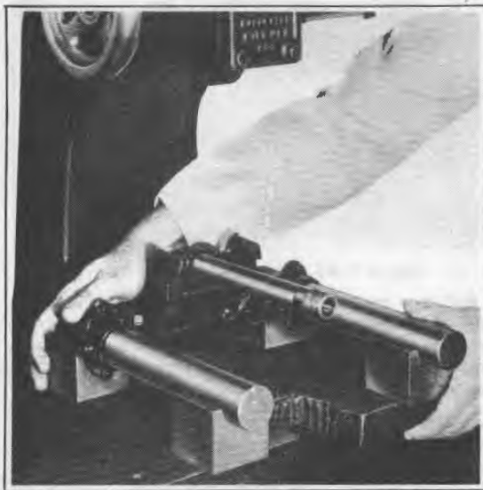
Figure 2-51. Checking Bracket Alignment
