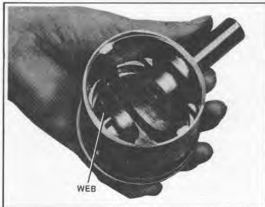
Figure 3-19. Piston with Web on Right Side
