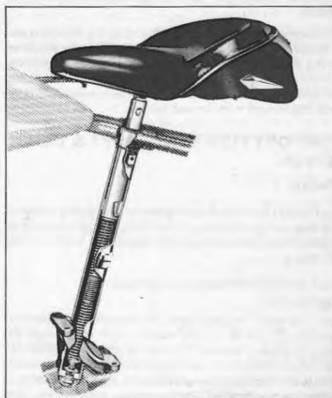
Figure 2-70. Cutaway of Seat Post Springing
