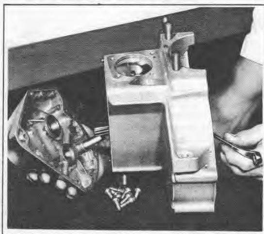
Figure 3-32. Line Reaming Cover Bushing
