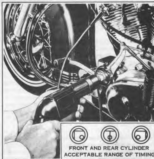
Figure 5-19. Checking Timing with Strobe Light
