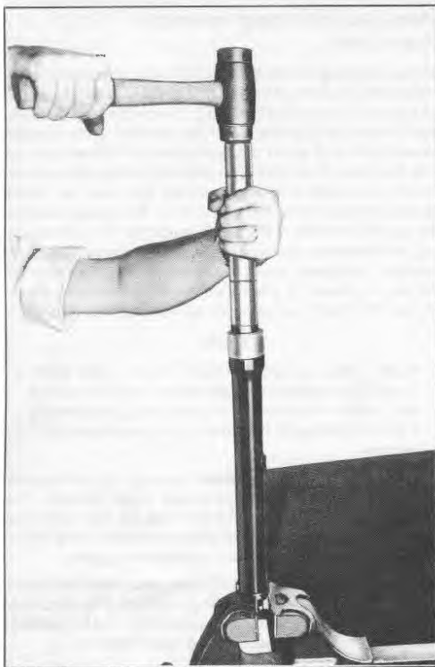
Figure 2-44. Installing Fork Slider Bushing
