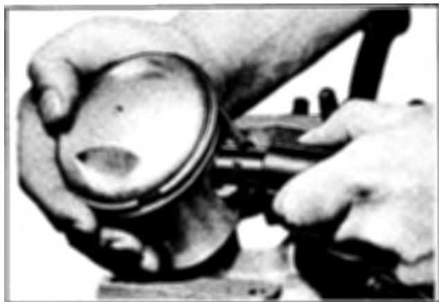
Figure 3-20. Inserting Piston Pin Lock Ring
