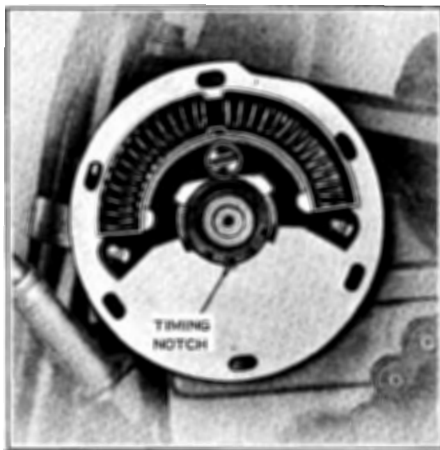
Figure 4-14. Timing Shifter Notches
