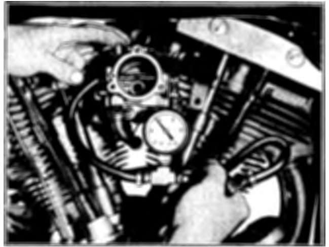
Figure 3-57. Checking Inlet Needle and Seat for Leakage
