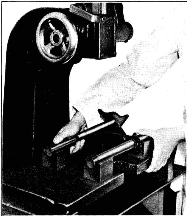
Figure 2-34J. Checking Bracket Alignment
