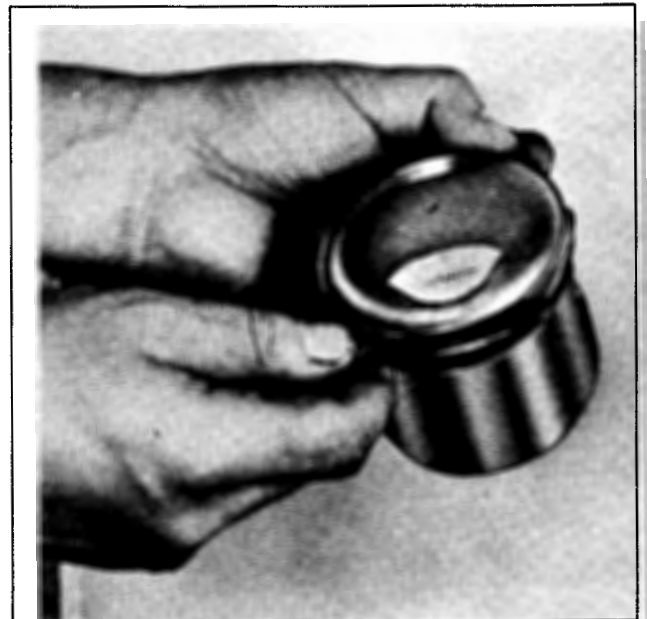
Figure 3-13. Measuring Ring Side Clearance
