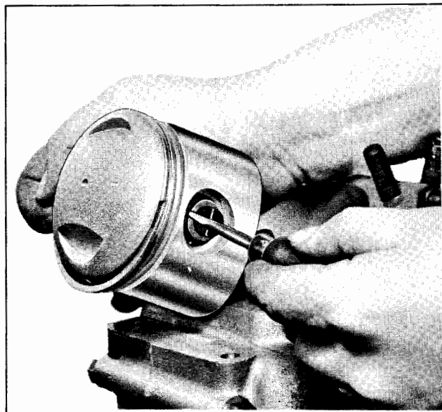
Figure 3-9. Removing Piston Pin Lock Ring
