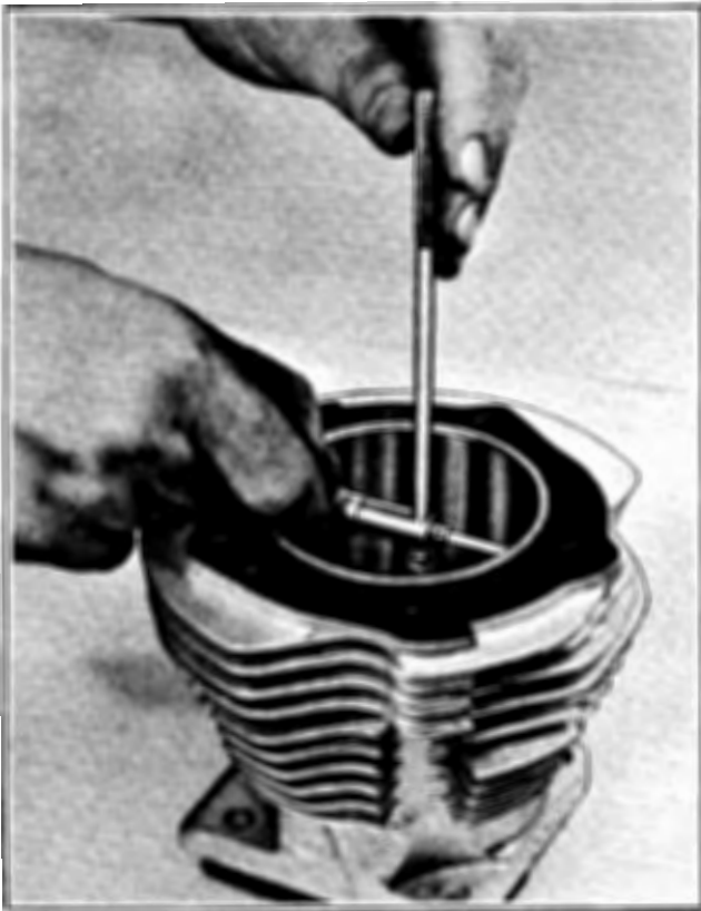
Figure 3-11. Measuring Cylinder Bore
