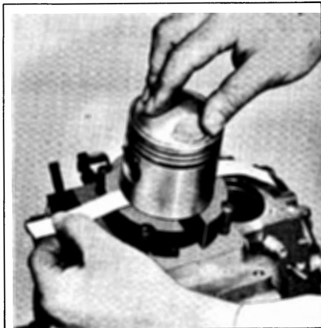
Figure 3-17. Checking Rod Alignment
