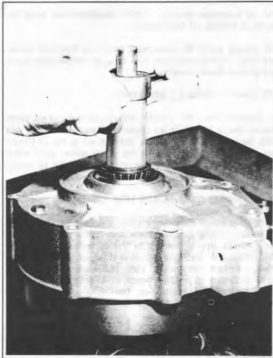
Figure 3E-17. Pressing Flywheel into Crankcase
