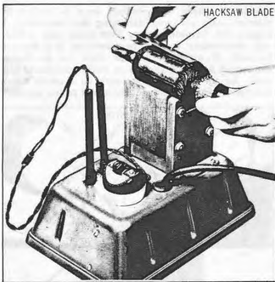
Figure 5E-4. Testing Armature for Short
