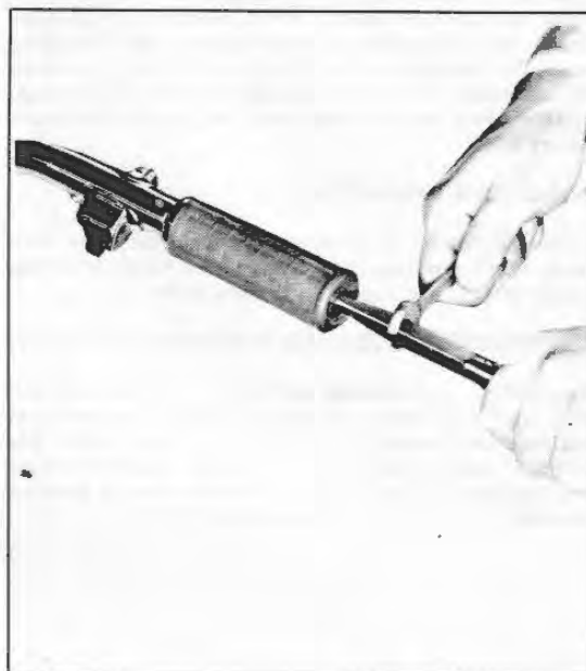
Figure 2D-1. Removing Handlebar Controls
