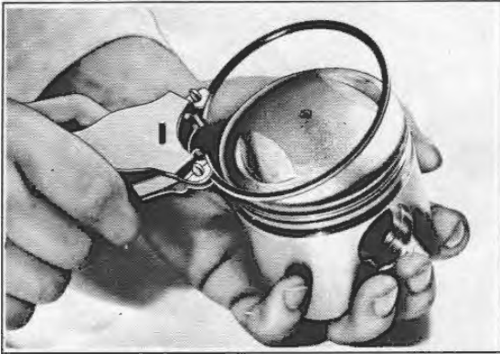
Figure 3C-9. Assembling Rings with Ring Expander
