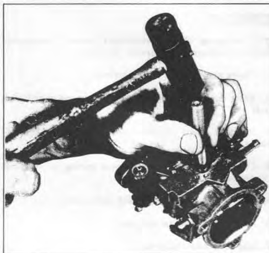
Figure 3F-7D. Removing Main Nozzle
