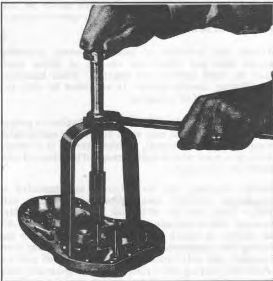
Figure 3D-6. Removing Pinion Shaft Cover Bushing
