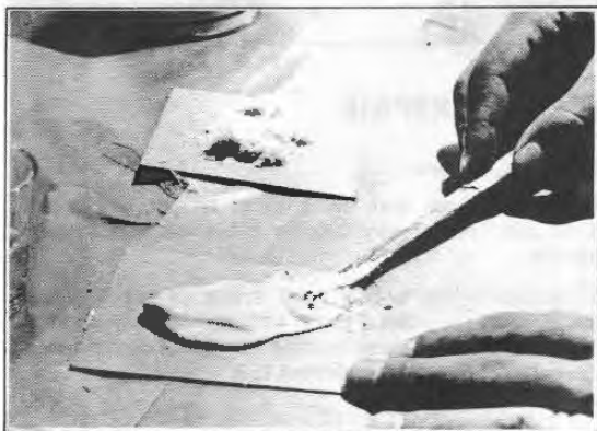
Figure 2J-2. Mixing Gel Coat and Glass Fibers
