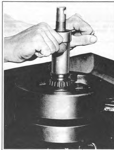
Figure 3E-16. Pressing Bearing on Sprocket Shaft
