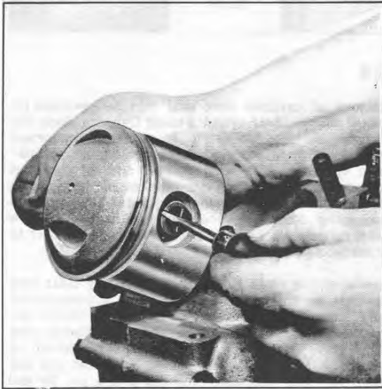
Figure 3C-2. Removing Piston Pin Lock Ring
