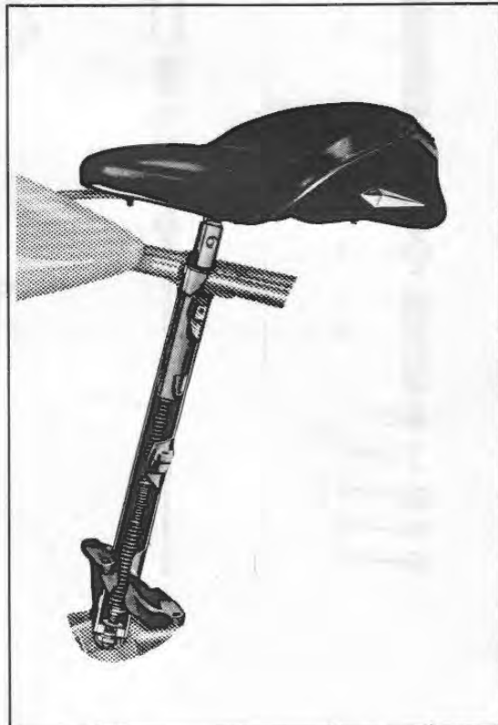
Figure 2H-1. Cutaway of Seat Post Springing
