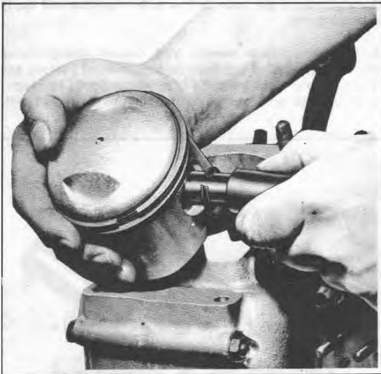
Figure 3C-14. Inserting Piston Pin Lock Ring
