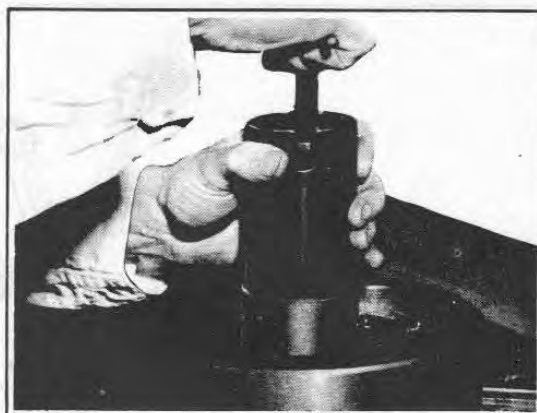
Figure 3E-7. Pulling Bearing from Sprocket Shaft
