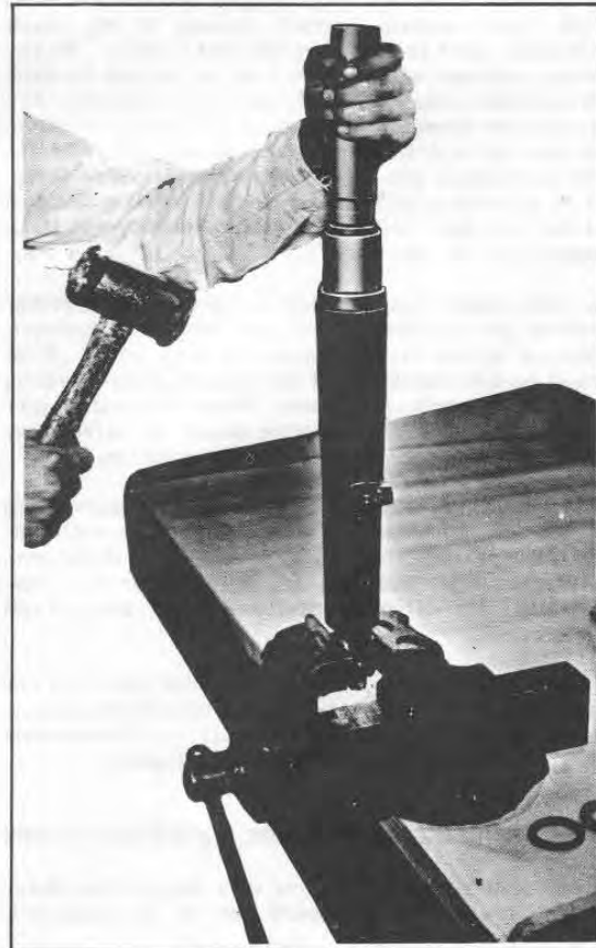
Figure 2F-7. Driving in Fork Slider Bushing
