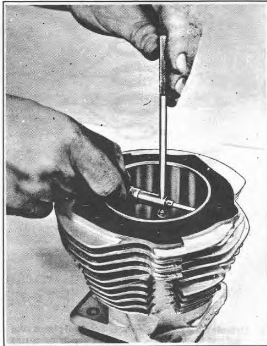
Figure 3C-4. Measuring Cylinder Bore
