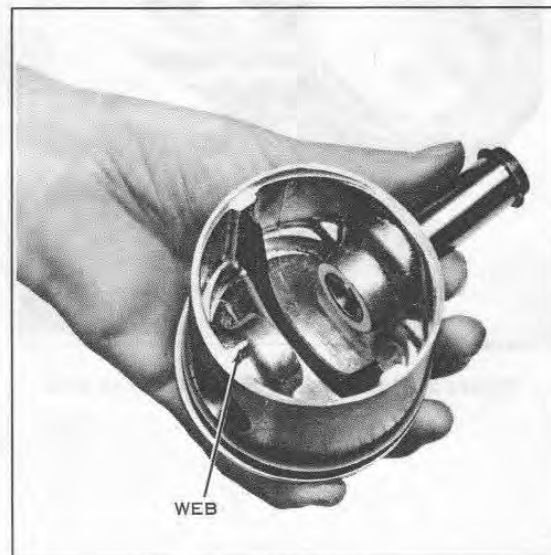
Figure 3C-13. Piston with Web on Right Side
