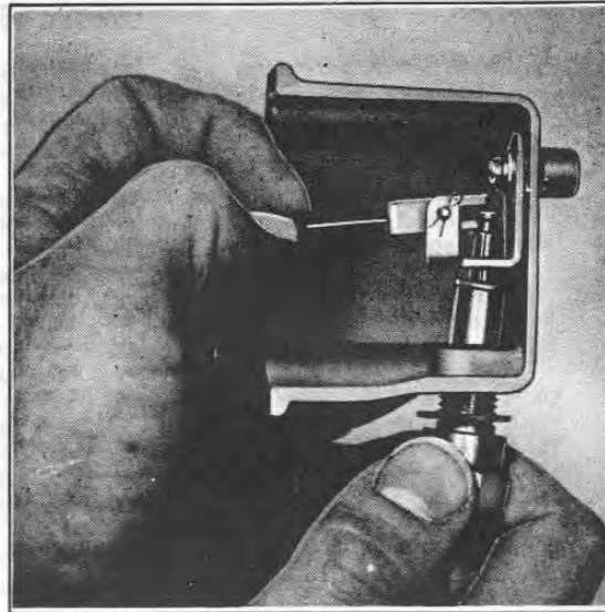
Figure 3F-9F. Engaging Model DC Float Lever in Valve Stem Groove
