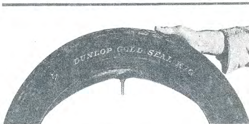
FIG. F.20. Cover and tube assembled ready for fitting.
