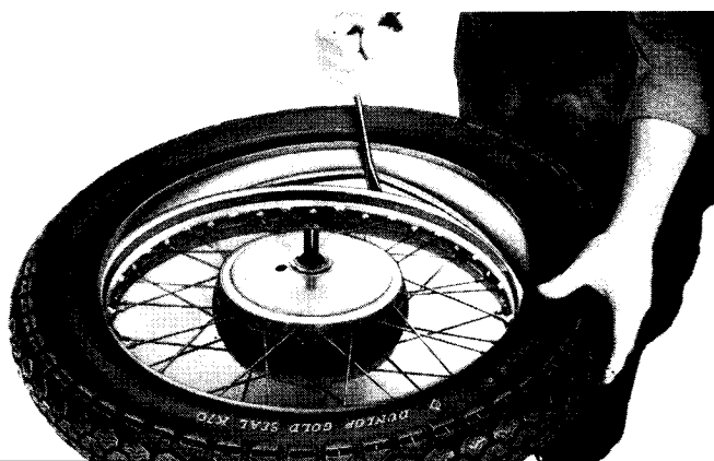
FIG. F.26. Completing the fitting of the first bead.
