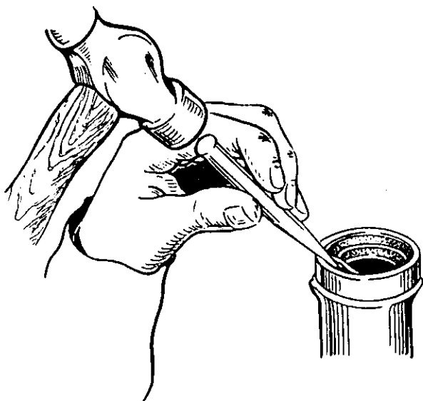
Fig. E5a. Removing the oil seal.
