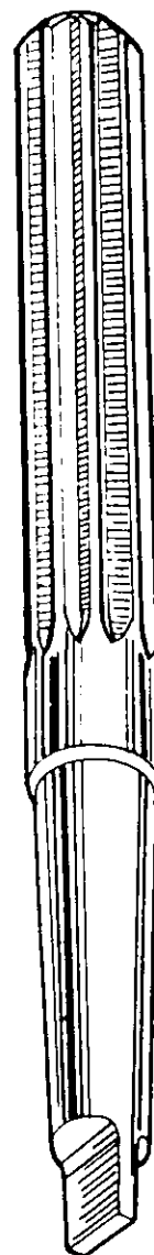
FIG. K.21. Reamer for top gear bush No. 61-6010.
