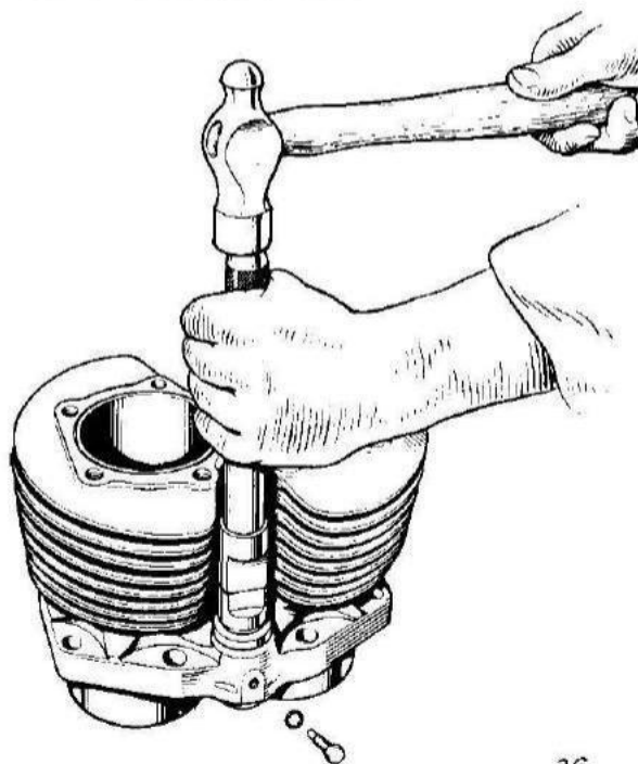
Fig. B18. Refitting a tappet guide block
