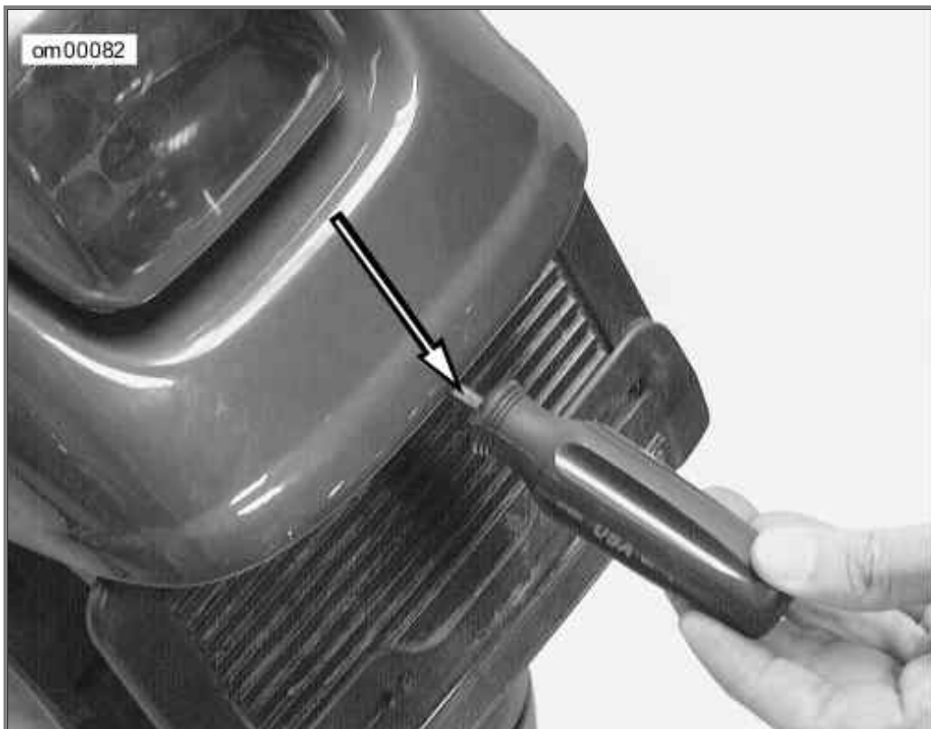
Tail Lamp Removal Access Hole: FXSTD Models
