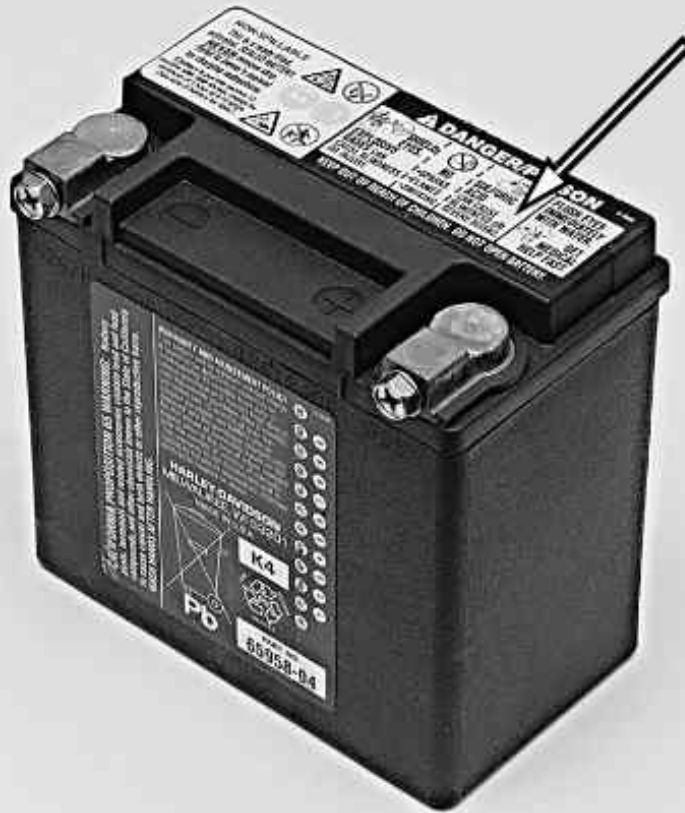
Battery Warning Label
