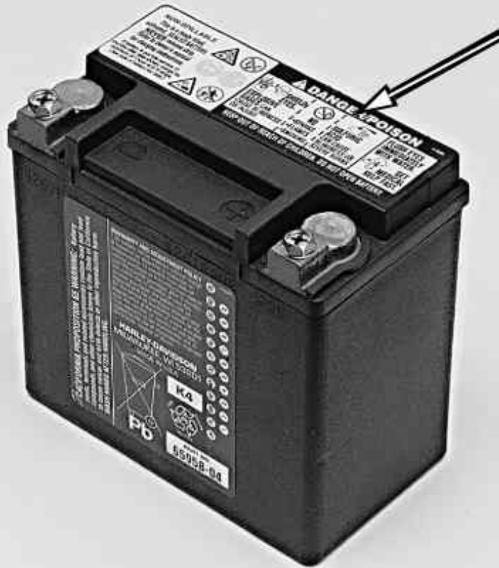
Battery Warning Label
