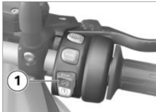
1 Emergency off switch (kill switch)
