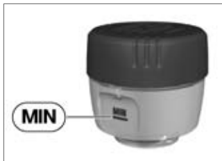
Brake fluid level, front
