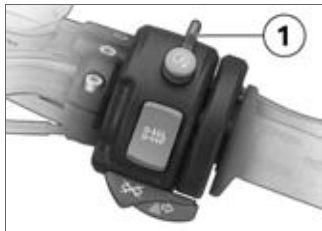
1 Emergency off switch (kill switch)
