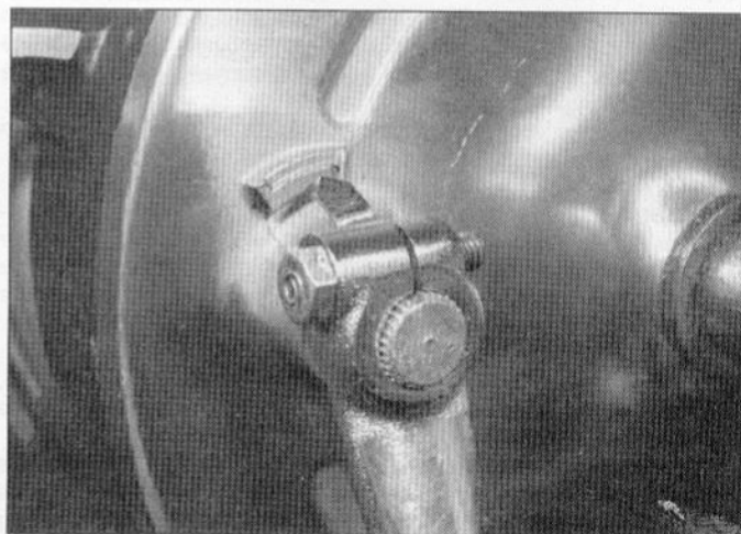
6.1 If the rear brake shoe indicator pointer moves past the end of the "safe movement" area on the scale, the shoes are worn and should be replaced
