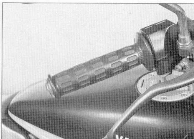
10.2 Twist the throttle grip lightly and check freeplay
