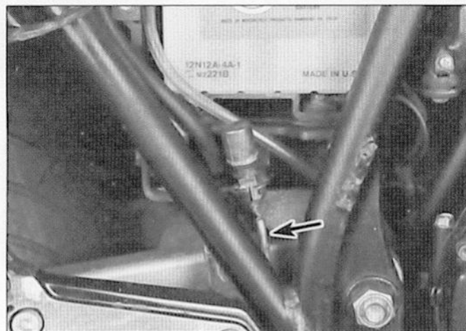
11.10 Disconnect the spring (arrow), unplug the electrical connector and rotate the plastic nut to remove the switch
