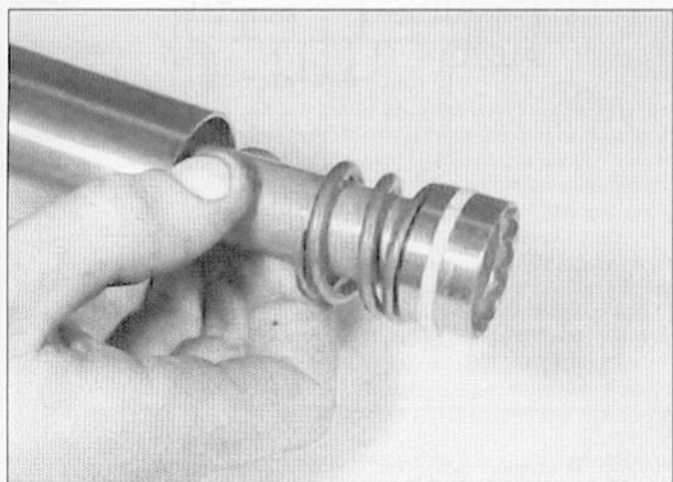
6.5 Remove the damper rod and the Teflon ring - don't separate the ring from the damper rod unless you plan to replace it
