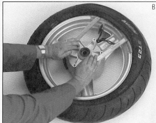
Use two levers to work bead over edge of rim. Note use of rim protectors.
