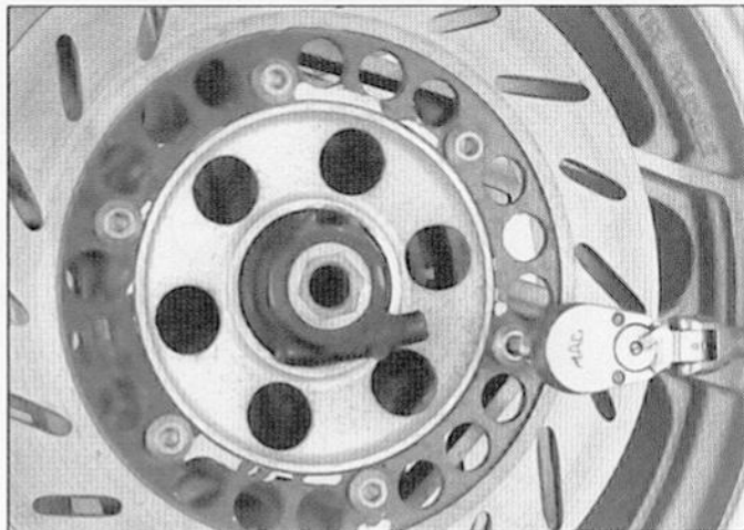
4.6 Loosen the mounting bolts evenly to detach the brake disc from the wheel
