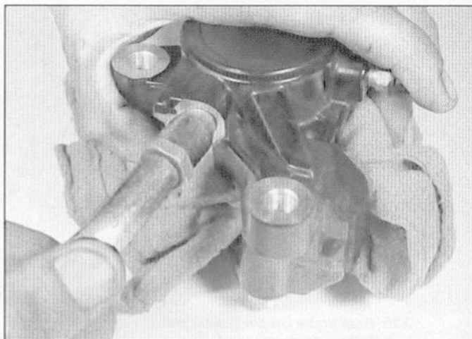
3.6 Blow air into the bleed valve hole to force the pistons out, but DO NOT get your fingers in the way
