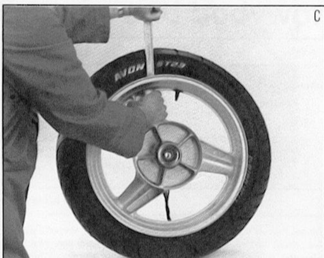
When first bead is clear, remove tire as shown.
