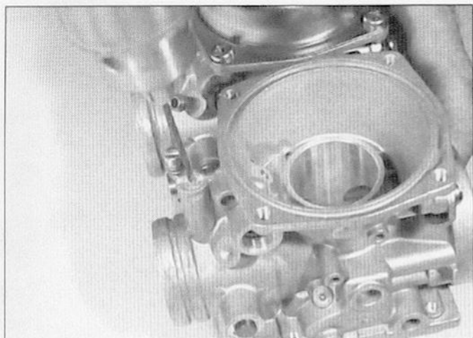
7.18a Drill out the pilot screw plug, but be very careful not to drill into the screw
