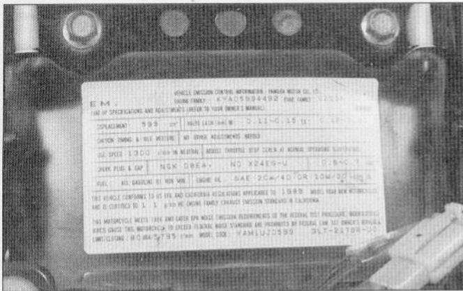
2.3a Maintenance information printed on decals includes tune-up and lubrication data . . .
