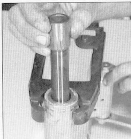
12.3 ... then pull out the bushing ...
