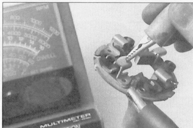
25.10 There should be no continuity between the brush plate and the brush holders (the resistance reading should be infinite)
