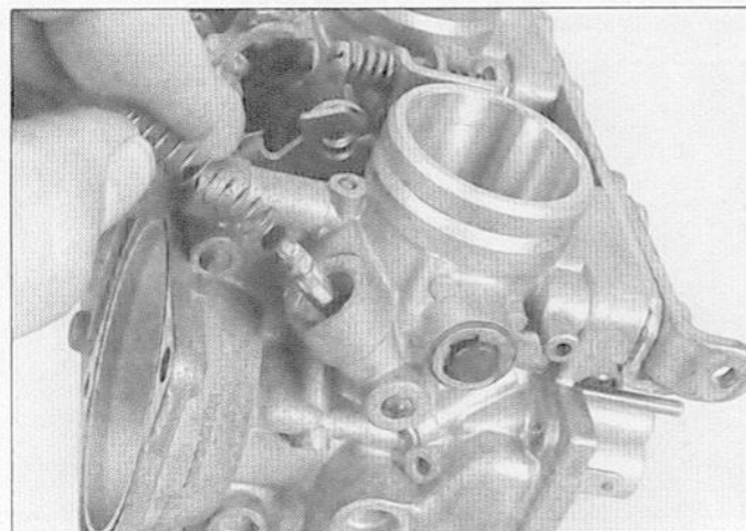
7.17b . . . and pull out the spring . . .
