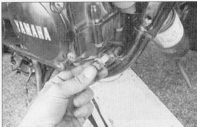
5.16b Pull the front bolts out once the nuts are removed . . .
