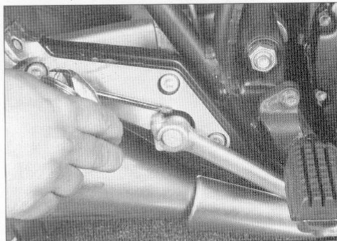
17.2d Lubricate the rear brake pedal at its pivot point
