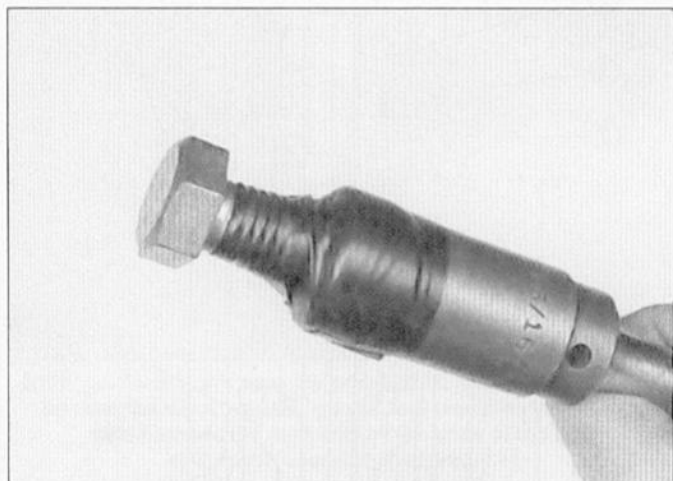
6.4e ... then install the nut-end into a socket (connected to a long extension) and tape it into place
