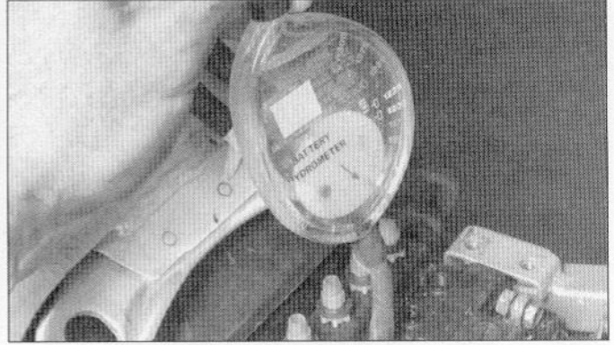
4.7 Check the specific gravity with a hydrometer
