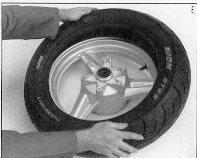
Work first bead over the rim flange.
