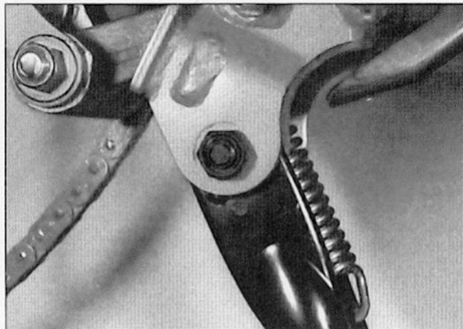
3.1 The centerstand pivots on two bolts
