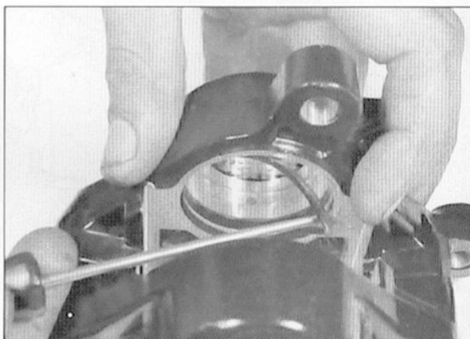
3.8b Remove the dust seal from its groove ...
