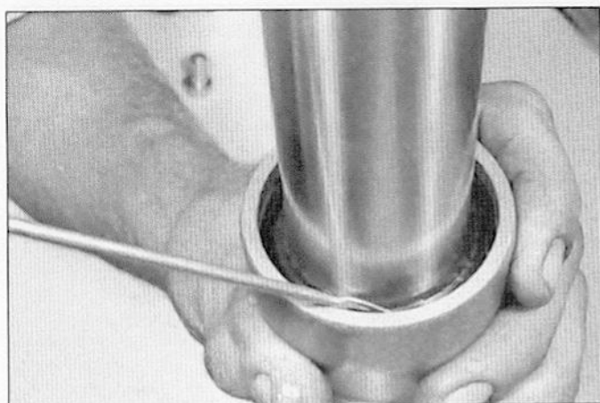
6.7 Pry out the retaining ring
