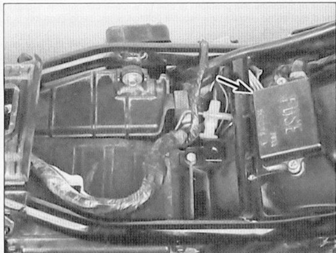
5.1a The fuse block is located under the seat (arrow) . . .
