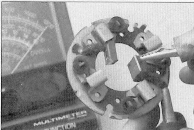
25.9 There should be almost no resistance (0 ohms) between the brushes and the brush plate
