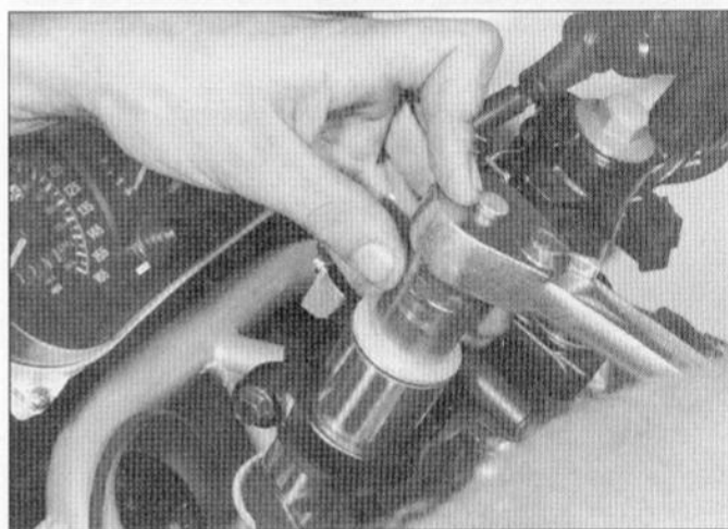
27.11 Unscrew the fork cap bolt . . .
