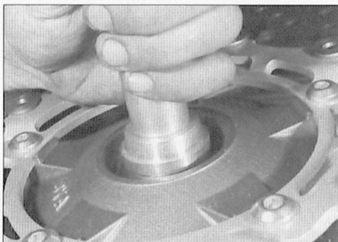
14.10 Install the bearing with a drive (shown) or a socket the same diameter as the bearing outer race
