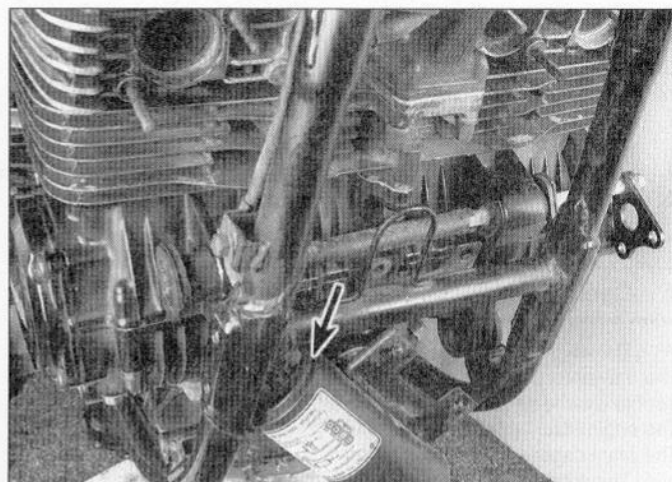
5.12 Unbolt the carbon canister and tie it out of the way (California models only)
