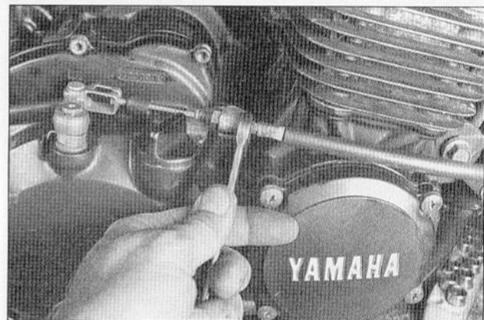
20.2 Loosen the nuts and detach the clutch cable from the bracket
