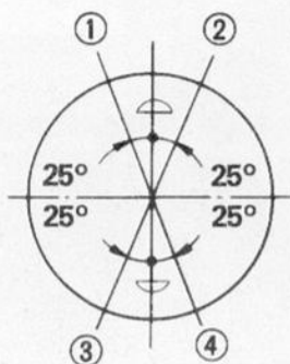
15.15 Arrange the ring gaps like this
