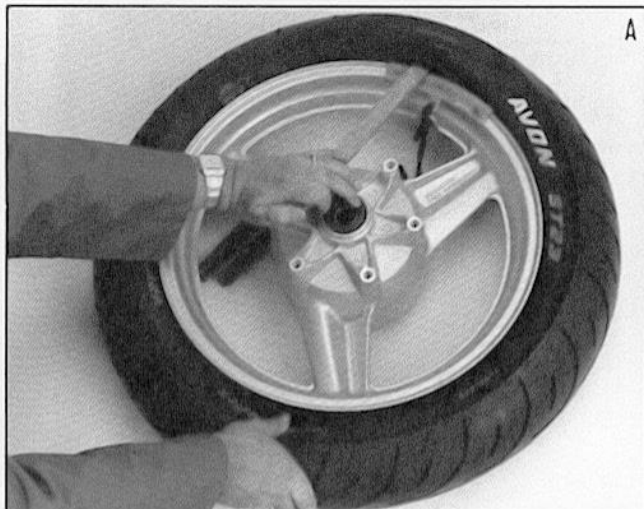
Deflate tire. After releasing beads, push tire bead into well of rim at point opposite valve. Insert lever next to valve and work bead over edge of rim.
