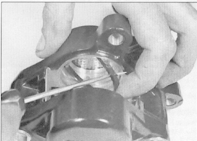
3.9 ... then remove the piston seal
