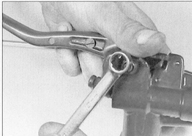
5.6 Remove the locknut and pivot bolt (master cylinder removed for clarity)
