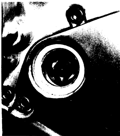
Clutch adjuster screw and locknut
