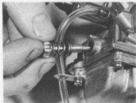
5.9a Remove and examine throttle stop ...
