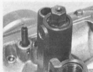
5.4b Main jet is a screw fit into needle jet ...
