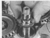
41.1b ... followed by a thrust washer
