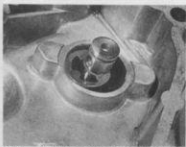
14.9b ... and secure it with a circlip as shown
