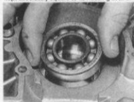
32.2 Heat crankcase casting before fitting bearings, taking care to prevent scalding the hands
