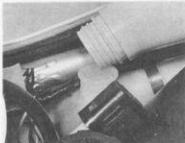
If level is low top up expansion tank
