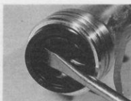
3.7a Use a large flat-bladed screwdriver to lever out oil seal ...
