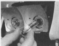
14.6f ... and uses a twin bulb arrangement. Note offset pins on bulb
