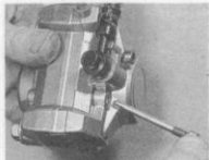
... and slacken and remove pad retaining bolts
