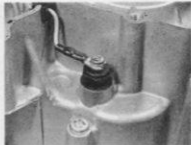
14.5a Neutral switch lead must be disconnected ...
