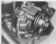
14.4 Pump is retained by two crosshead screws
