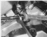
4.9 Slacken clutch cable adjuster and disconnect cable
