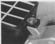
4.2b ... then remove mounting bolt and remove complete air filter assembly from machine
