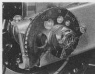
5.6 Ensure snail cam adjusters are fitted as shown
