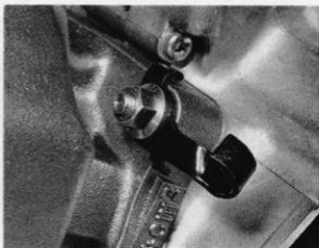
44.4b Do not forget clutch cable bracket when refitting barrel retaining nuts
