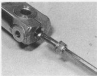
3.9d Apply thread-locking compound to damper rod Allen bolt and tighten to specified torque setting
