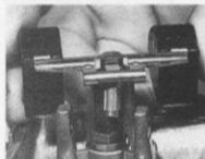
5.2d ... and remove float assembly and needle for examination
