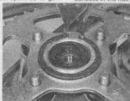
7.2b ... followed by large circlip ...
