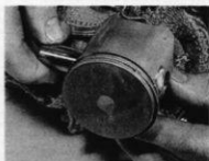
44.3 Fit piston ensuring that arrow on piston crown faces forwards
