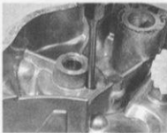
9.4a Drift out water pump seal via hole provided in crankcase cover
