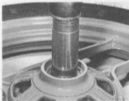
6.8c ... using a hammer and tubular drift
