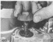
9.5 Grease impeller spindle and oil seal lip before fitting impeller
