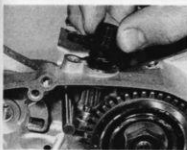
39.1a Fit driven gear and plastic housing. Avoid overtightening the retaining bolt
