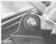
4.7b ... and remove rear mounting bolt
