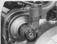
4.10 Remove kickstart lever, marking its shaft if necessary
