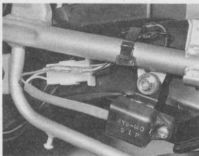
9.1 Ignition control unit location - TZR 2RK and 3PC1 models
