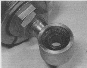
14.4 Examine suspension unit bushes for wear or corrosion - renew if necessary
