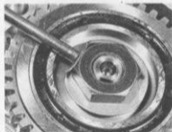
38.4b ... and tighten nut to specified torque setting - secure with the tab washer
