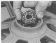
6.8b ... and fit second bearing ...
