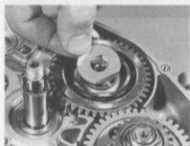
38.4a Fit a new tab washer ...
