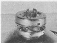
14.3b ... then bulbholder ring ...
