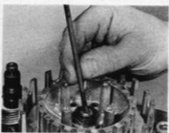
41.3b Grease clutch left-hand pushrod and insert it into input shaft ...
