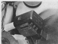
11.1a The turn signal relay is situated between oil and expansion tanks on TZR model ...
