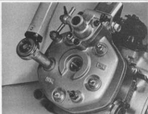
44.5b ... and tighten cylinder head nuts to specified torque settings
