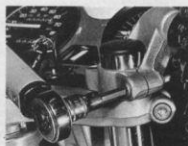
2.3b ... and clip-on handlebars must first be removed
