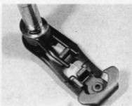
37.2 Ensure gearchange shaft return spring is correctly fitted
