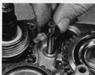
39.1b Fit a plain thrust washer ...
