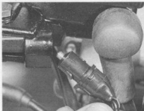
8.6 Remove front stop lamp switch as described in text
