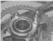
7.2a TZR model - remove sprocket retaining nuts and tab washers ...
