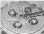
If necessary, adjust clutch release mechanism (see text) ...
