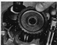
40.1b ... followed by first plain thrust washer and idler gear
