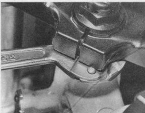
8.3 Use a C-spanner to adjust steering head bearings
