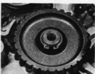
40.1c Fit second plain thrust washer and secure with another circlip
