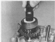
40.3a Install kickstart assembly ensuring friction clip is correctly located in recess provided in casing ...
