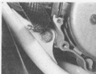
4.18a DT125 - remove top engine mounting bracket and front mounting bolt ...
