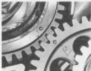
38.3c ... and rotate gear until both punch marks align
