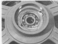
6.8a TZR model - fit speedometer drive ring as shown ...
