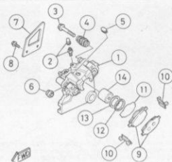
Fig. 6.10 Rear brake caliper - DT model
