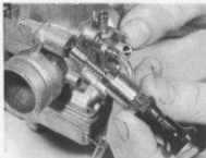
5.8 Choke assembly is screwed into the carburettor body – early type carburettor shown
