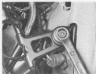
14.2a Release headlamp unit by removing the bolts (DT model) ...
