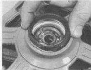
6.8c Grease seal to aid installation
