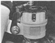
...and rear master cylinder reservoirs - ensure level does not fall past lower mark
