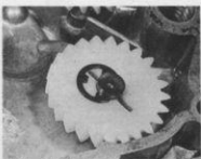
14.9d ... and nylon drive gear - secure with the second circlip
