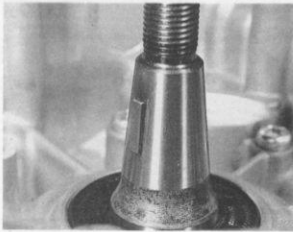
36.1 Fit Woodruff key to the crankshaft ...
