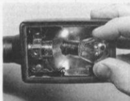
14.6c Turn signal bulbs are a bayonet fit in their holders
