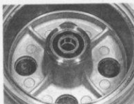
8.4a Cush drive bushes can be driven out via access holes in opposite side of hub...
