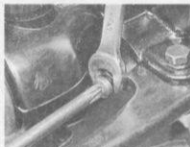
Adjust front brake lever free play using screw and locknut
