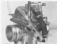
5.2a Disconnect power jet pipe and remove float chamber retaining screws ...
