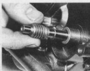
14.9a Insert drive shaft ...
