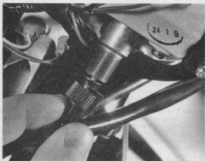
17.2b Release drive cables ...
