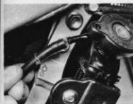
5.2a Disconnect expansion tank hose from radiator neck ...
