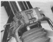
2.4b ... and bottom yokes to release fork legs – DT model shown
