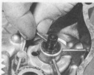
9.6a Refit first plain washer and secure it with locating pin
