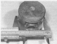
24.2 Measuring piston outside diameter
