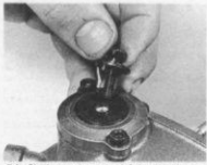
7.3a Slacken and remove left-hand valve cap centre bolt followed by the valve cap itself ...
