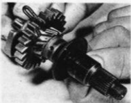
40.2b Slide large plain washer into position
