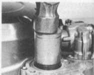
9.4c If necessary drift seal into position using a suitably sized socket
