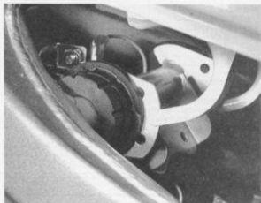
2.6 On refitting ensure tank engages correctly with rubber buffers - TZR model shown
