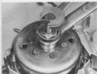
14.4 Extractor must be used to remove rotor
