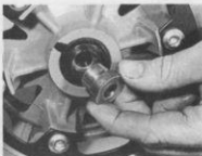
3.1b ... and spacer - TZR model shown
