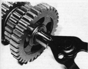
30.8j Secure with a thrust washer and circlip
