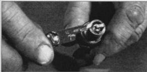
Electrode gap check - use a wire type gauge for best results
