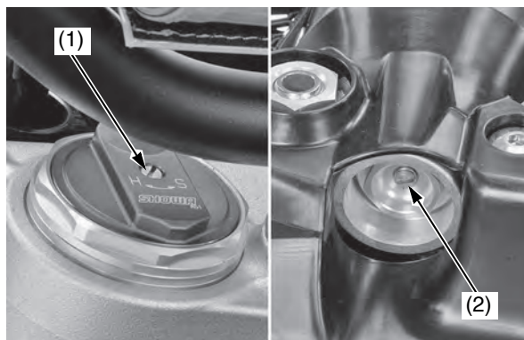
(1) compression damping adjuster (2) rebound damping adjuster
