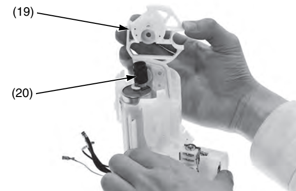
(19) fuel pump stopper (20) damper rubber
