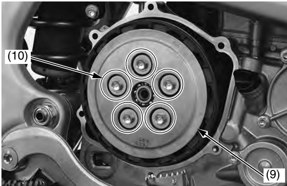
(9) clutch pressure plate (10) clutch springs and bolts
