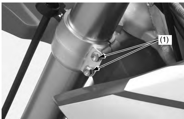
(1) fork bridge lower pinch bolts
