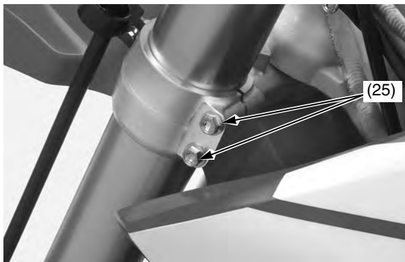
(25) fork bridge lower pinch bolts
