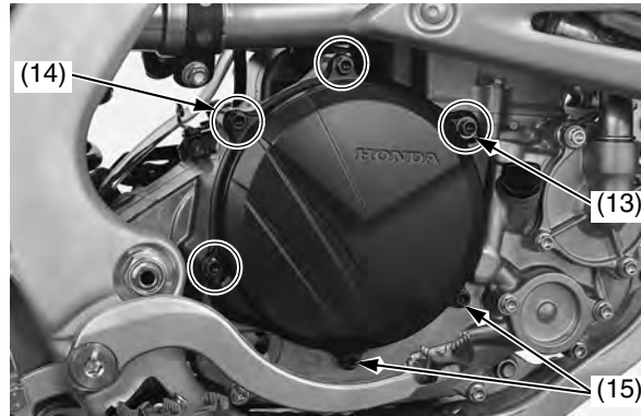
(13) washer (new) (14) clutch cover A bolts (15) clutch cover B bolts
