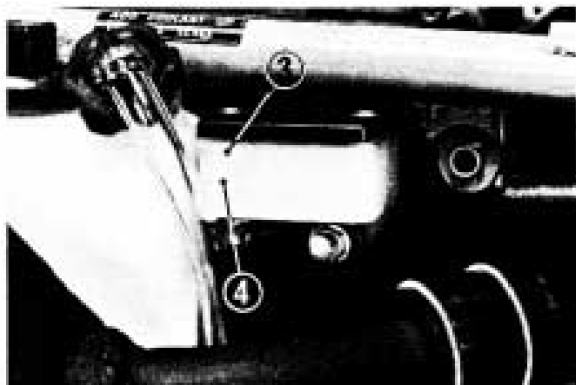
(REAR) (3) Upper level mark (4) Lower level mark
