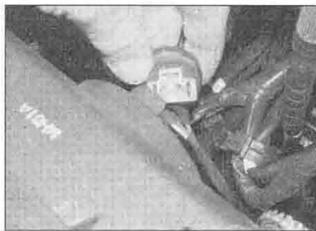
7.2b Disconnect the wiring connector – XL650V
