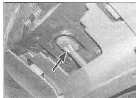
7.8a Sidelight bulbholder (arrowed) - XL650V
