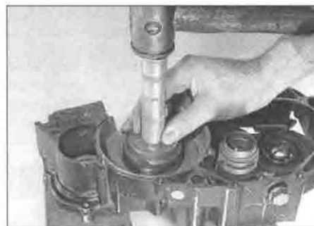
5.1 Using a bearing driver against the bearing's outer race
