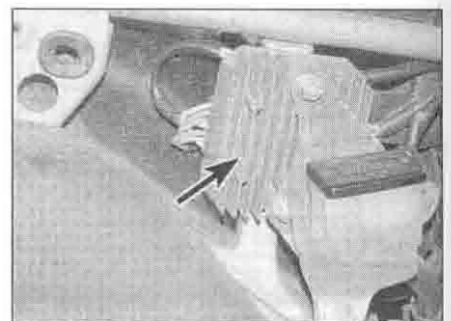
33.1a Regulator/rectifier (arrowed) – XL600V
