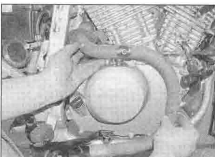
13.4b ... and remove the downpipe
