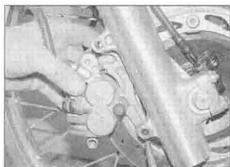
4.19 Slide the caliper onto the disc and install the bolts
