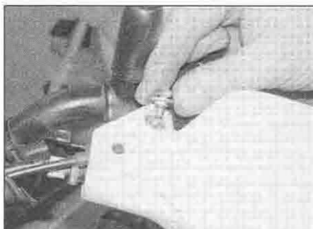
5.15a Unscrew the bolt and remove the collar
