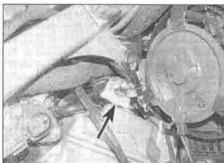
3.18d Front cylinder HT coil (arrowed) - XRV single coil per cylinder models
