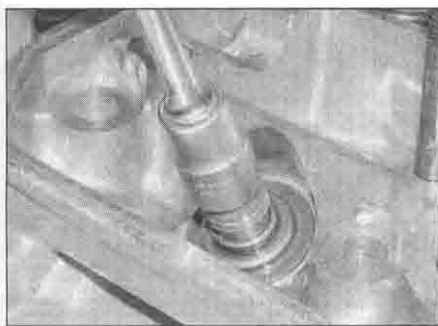
14.26b ... using a deep socket or special tool to press it squarely into place
