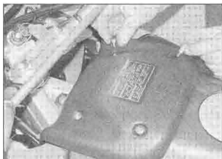
2.17a Undo the screws . . .
