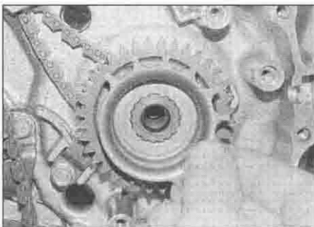
21.8 ... and on XL models the timing rotor
