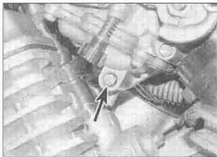
7.9a Carburettor drain screw (arrowed) – XL models
