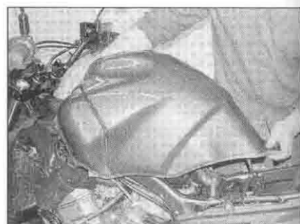
2.12 Carefully remove the tank
