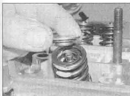
14.28c ... then fit the spring retainer
