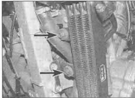
7.3 Oil cooler mounting bolts (arrowed)
