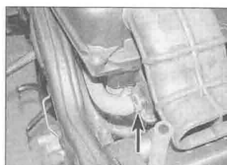
4.5a Detach the hose (arrowed) from its union
