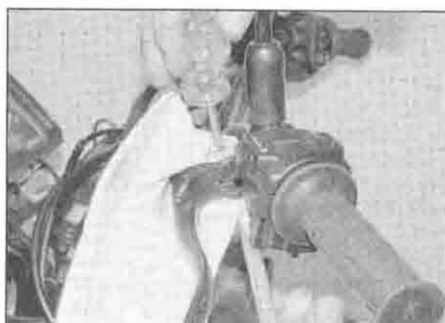
12.3b Counter-hold the screwhead and undo the nut on the bottom ...
