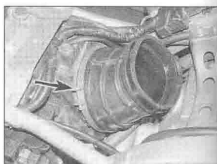
4.2e Slacken the clamp screw (arrowed) and remove the joint piece if required
