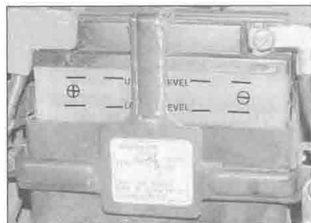
6.2 Make sure the level in each cell is between the UPPER and LOWER level lines
