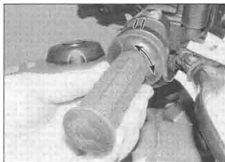
15.3 Throttle cable freeplay is measured in terms of twistgrip rotation
