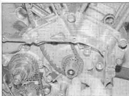
10.14a Slide the sprocket out and remove the chain ...
