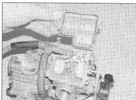
10.9 Fit a new O-ring into the groove and install the float chamber
