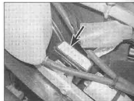
5.3c Fusebox (arrowed) – XRV750-P models on
