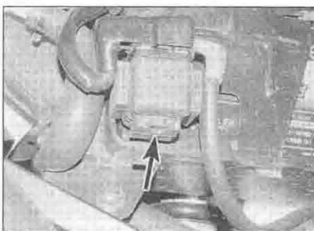
5.5 A spare main fuse (arrowed) is housed with the relay
