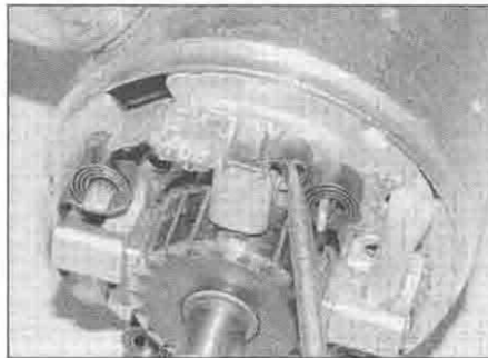
29.17 Locate the spring ends onto the brushes
