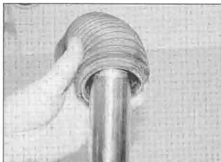
8.2 Remove the gaiter
