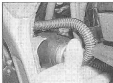
11.10a On XRV750 models displace the fuel pump from its mount
