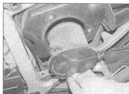
8.1b ... and withdraw the filter
