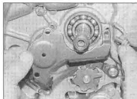
20.4c Unscrew the remaining bolts and remove the retainer plate
