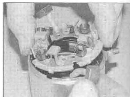
29.7b Remove the brushplate assembly ...
