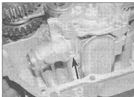
25.2a Unscrew the bolt (arrowed) ...
