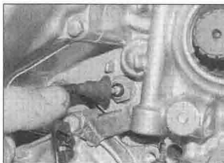
5.17a Detach the neutral switch wiring connector ...
