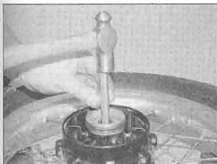
15.17 Drive the bearings out as described
