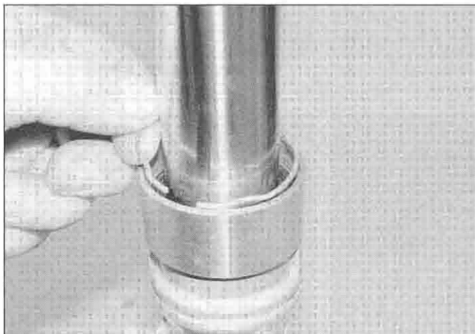
8.24 Install the retaining clip ...
