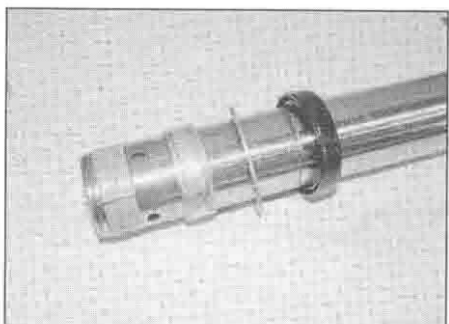
8.11b ... the slide-hammer effect will displace the oil seal and bush
