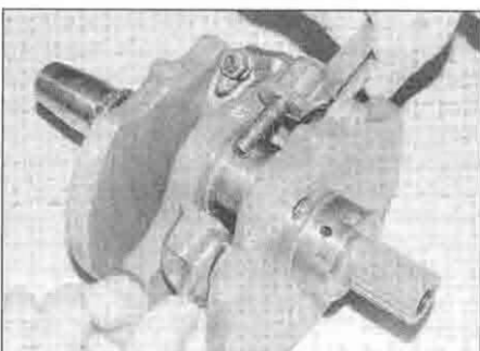
28.4b ... and separate the rod from the shaft
