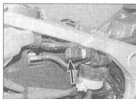
25.2c Diode (arrowed) – XRV750
