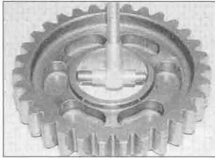
31.20a Measure the internal diameter of the gear ...
