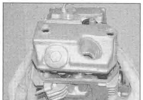
8.7 Lift the cover off the cylinder head
