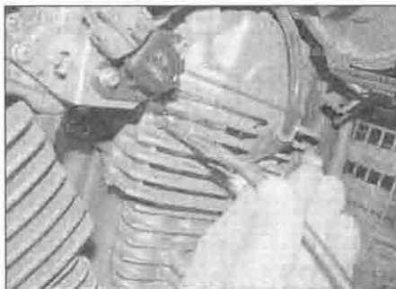
17.8 Connect the gauge hoses to the vacuum take-off points
