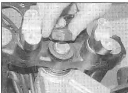
19.8b ... then unscrew the nut ...
