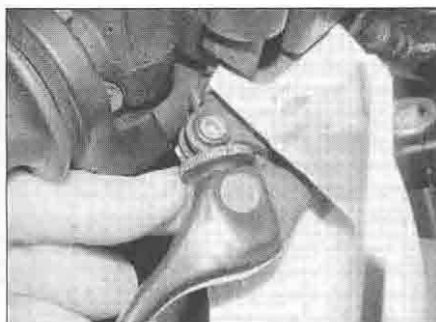
19.6 Adjusting the front brake lever span
