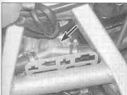
5.3c . . . to access the thermostat housing (arrowed)
