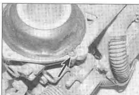
10.12b ... then press the diaphragm rim into the groove, making sure the loop (arrowed) locates correctly
