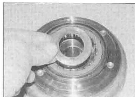
22.4b . . . and on XL models remove the thrust washer
