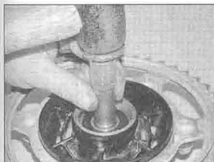
15.26 Drive out the spacer...
