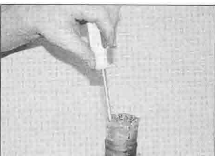
13.7a Dig out the old sealing ring ...
