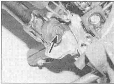
23.13 Sidestand switch mounting bolt (arrowed)
