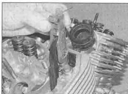
11.4b ... then withdraw the tensioner ...
