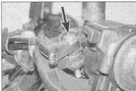
5.16 Undo the screw (arrowed), lift off the choke lever, slide out the clutch lever and detach the cable
