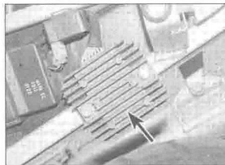
33.1c Regulator/rectifier (arrowed) - XRV750-P models onward (1993-on)
