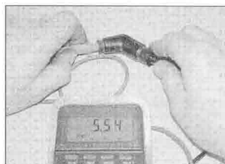
3.8 Measuring spark plug cap resistance
