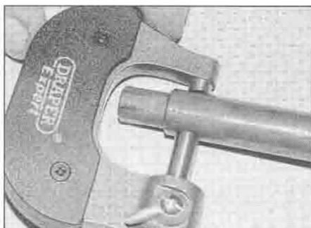
29.11b ... and the external diameter of its location on the shaft
