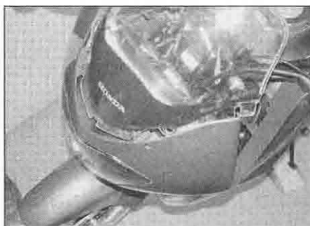
5.10b ... then remove the windshield
