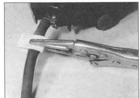
9.4 ... or thick card and self-locking grips
