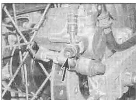
5.1a Brake hose banjo bolt (arrowed) – XL600V
