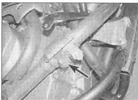
13.3a Slacken the clamp bolt (arrowed)
