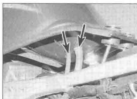
2.18b ... and the breather and overflow hoses (arrowed) – later model type shown
