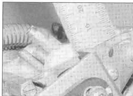
10.8 Measuring the float height
