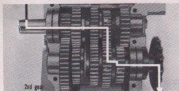
Fig. 4-105. Second gear (C4 is shifted)
