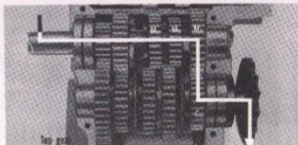
Fig. 4-108. Top gear (M2-M3 is shifted)
