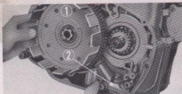
① Clutch outer ② Oil pump Fig. 4-71. Removing the clutch outer
