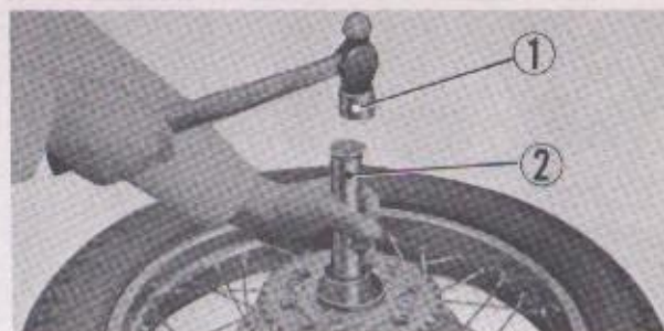
① Hammer ② Bearing driver Fig. 5-135. Installing the bearing
