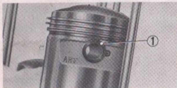
① Piston pin clip Fig. 4-56. Setting the piston pin clip
