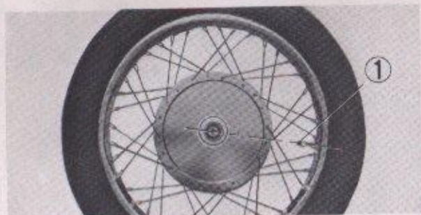
① Valve stem Fig. 5-89. Valve angle
