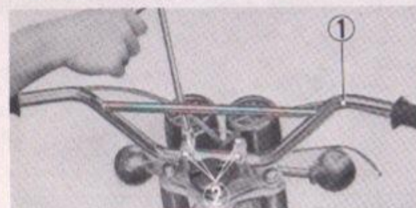
① Steering handle pipe ② 8mm hex. bolt
