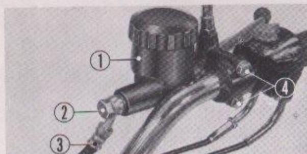
① Master cylinder body ② Joint bolt ③ Brake hose ④ Setting bolts Fig. 5-110.
