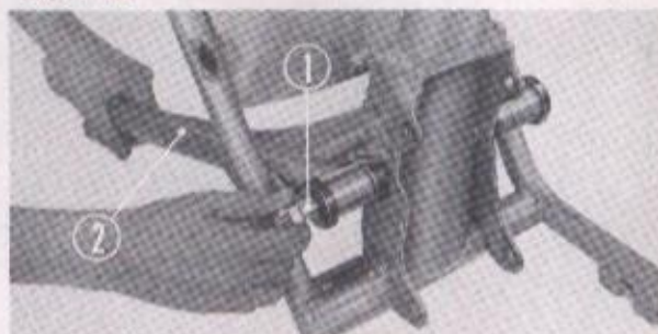
① Rear fork pivot bolt ② Rear fork
