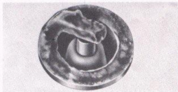
Fig. 6-24. Sooty condition (dry)
