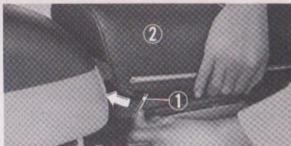
① Seat latch lever ② Seat
