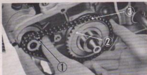
① Starting motor sprocket ② Starting sprocket ③ Starting chain
