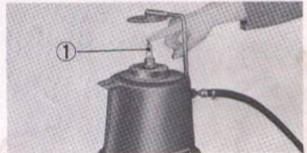
① Spark plug Fig. 6-27. Spark plug cleaning
