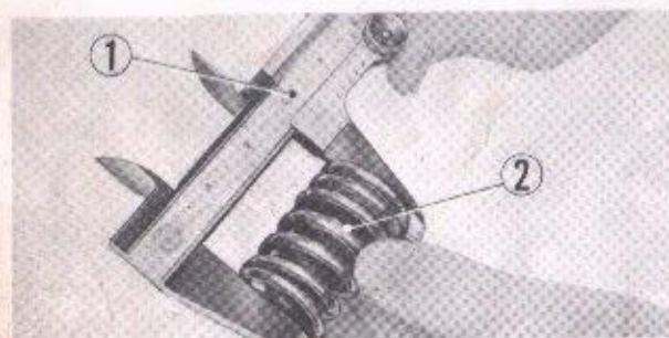
① Vernier caliper ② Clutch spring Fig. 4-89. Measuring free length of clutch spring
