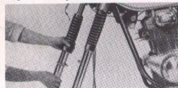
Fig. 5-27. Installing the front fork into the steering
