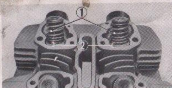
① Valve springs ② Smaller pitch Fig. 4-38. Installing valve spring
