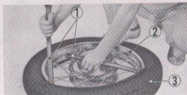
① Tire lever ② Rear wheel rim ③ Rear wheel tire Fig. 5-131. Removing the rear wheel tire
