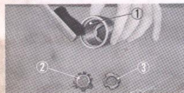
① Oil filter rotor ② Lock washer ③ Lock nut Fig. 4-75. Cleaning oil filter
