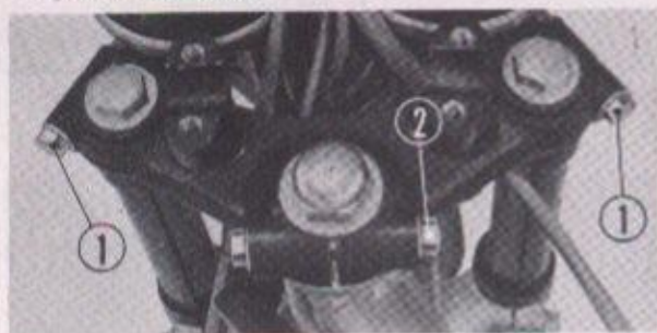
① Fork mounting bolt ② Steering stem setting bolt Fig. 8-2. Fork top bridge
