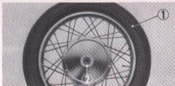
① Front wheel tire ② Oil-seal Fig. 5-82. Removing the oil-seal
