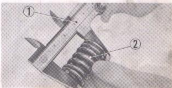
① Vernier caliper ② Valve spring
