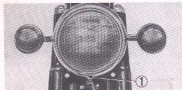
① Adjusting screw Fig. 6-71. Headlight (General export type)
