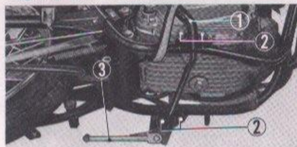
① Step bar ② 8mm bolts ③ Side stand
