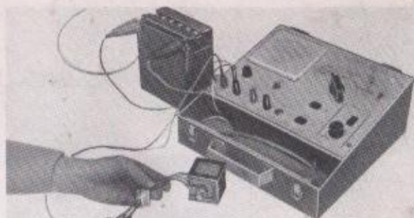
Fig. 6-40. Rectifier resistance measurement
