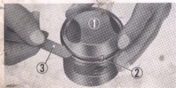
① Piston ② Piston ring ③ Thickness gauge Fig. 4-49. Piston groove and piston ring clearance
