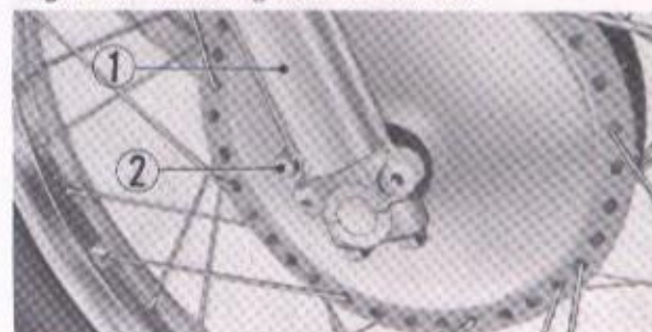
① Front fork bottom case ② Front fork drain plug Fig. 5-22. Removing front fork drain plug
