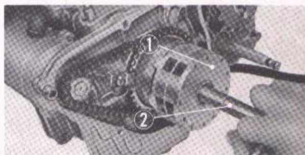
① Generator rotor ② Generator rotor puller Fig. 4-94. Removing the generator rotor
