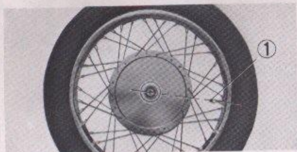
① Valve stem Fig. 5-89. Valve angle
