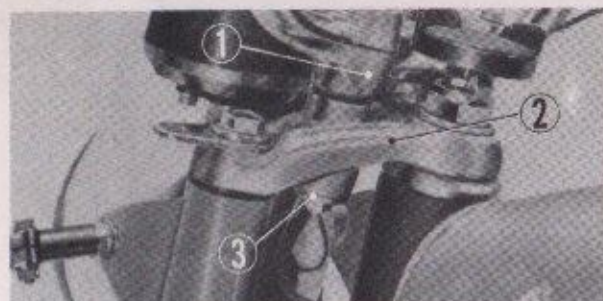
① Handle pipe under holder ② Fork top bridge ③ 8 mm nut
