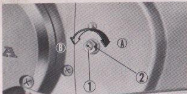
① Clutch adjusting screw ② Clutch adjusting screw lock nut Fig. 4-86.
