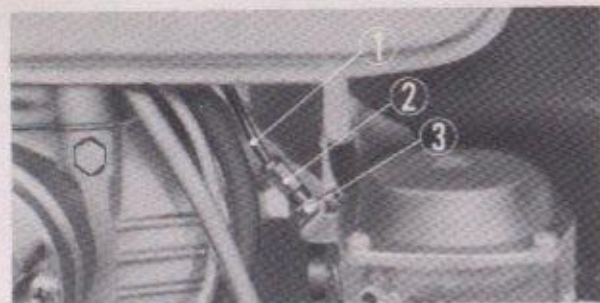
① Throttle cable ② Throttle cable adjuster ③ Lock nut
