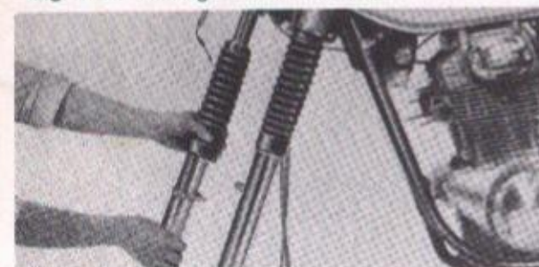
Fig. 5-27. Installing the front fork into the steering
