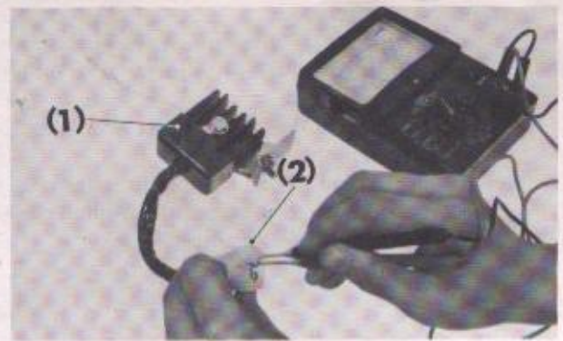
Fig. 5-14 (1) Silicon diode rectifier (2) Connector
