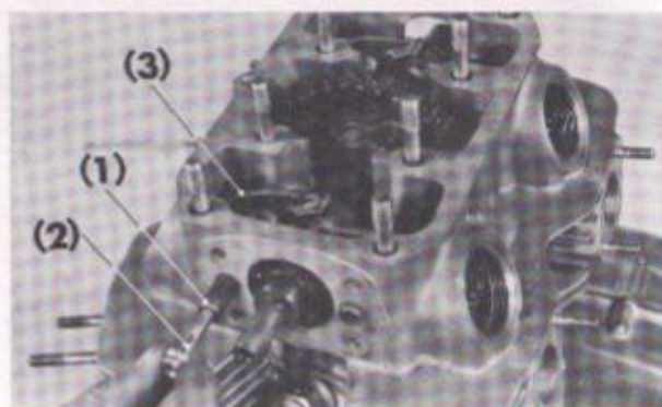
Fig. 3-4 (1) Rocker arm shaft (2) 6mm bolt (3) Rocker arm
