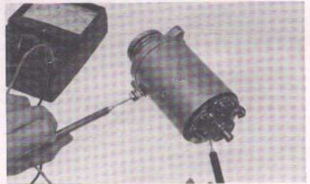
Fig. 5-24 Checking stator coil
