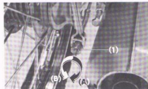
Fig. 2-23 (1) Rear brake adjusting nut
