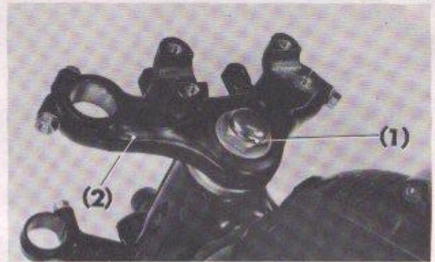
Fig. 4-58 (1) Steering stem nut (2) Fork top bridge
