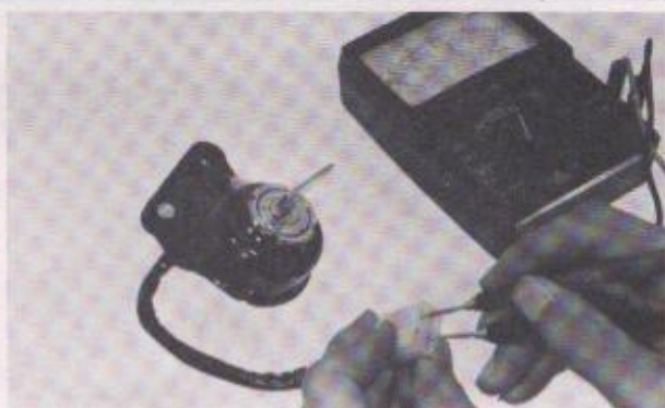
Fig. 5-29 Checking main switch for continuity
