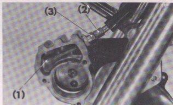
Fig. 4-22 (1) Cable end (2) Adjusting bolt (3) Brake cable bolt
