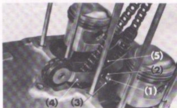
Fig. 3-55 (1) Bolt (2) Snap ring (3) Guide roller pin (4) Chain tensioner roller (5) Guide roller
