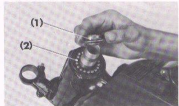
Fig. 4-60 (1) Top cone race (2) # 8 steel ball
