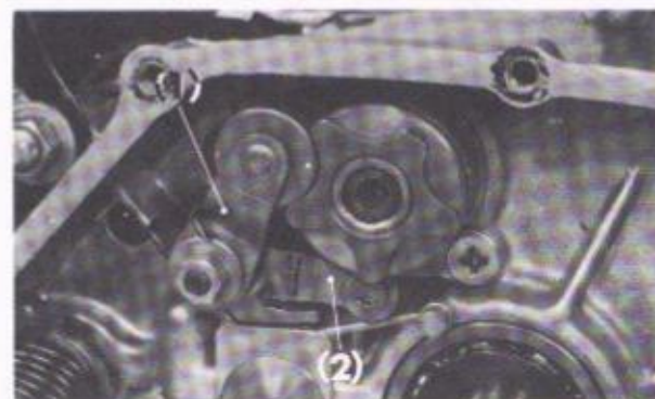
Fig. 3-45 (1) Gear shift drum stopper arm (2) Neutral stopper arm
