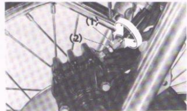
Fig. 4-29 (1) Cable adjusting bolt (2) Lock nut
