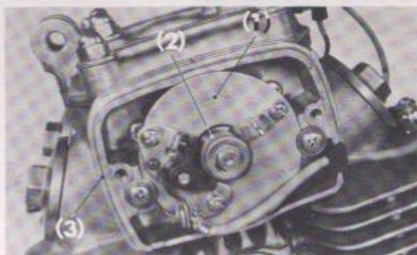
Fig. 3-3 (1) Contact breaker base plate (2) Spark advancer (3) Point base
