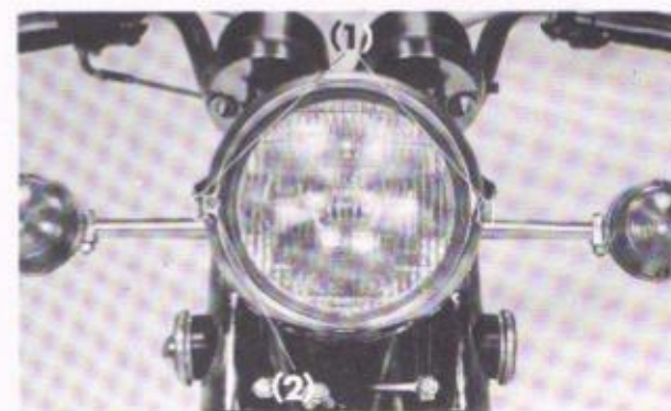
Fig. 2-39 (1) Headlight mounting bolt (2) Adjusting screw
