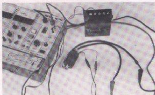
Fig. 5-4 Checking ignition coil performance
