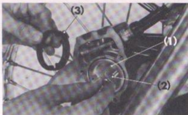
Fig. 4-15 (1) Pad A (2) 6mm bolt (3) Thrust plate guide
