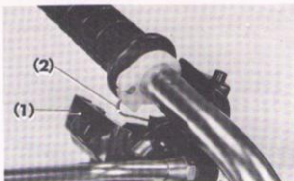
Fig. 4-49 (1) Switch (2) Throttle cable
