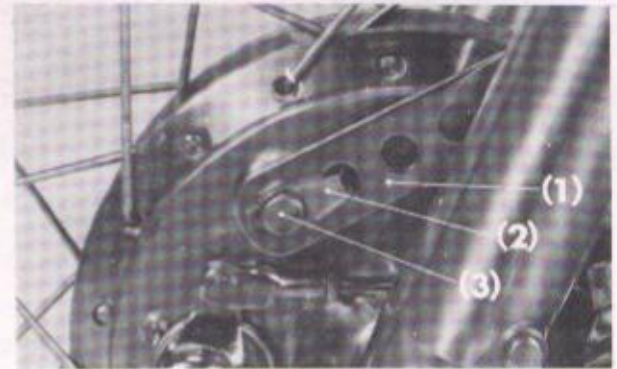
Fig. 4-40 (1) Brake stopper arm (2) Lock washer (3) Bolt
