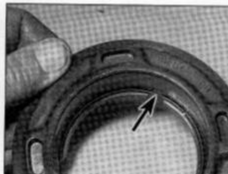
18.17b The spring seat (arrow) fits inside the pressure plate
