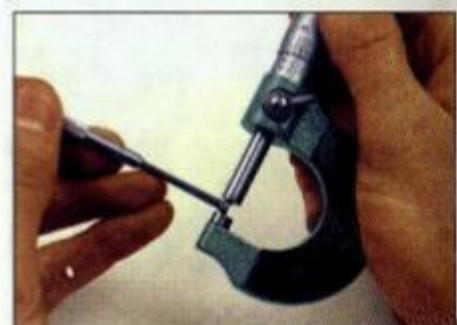
3.10 ... then measure the gauge with a micrometer
