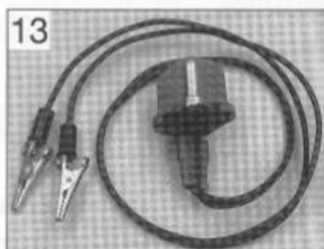
A buzzer is useful for voltage checks
