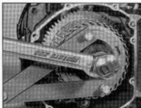
18.51c ... and tighten it to the specified torque setting, using the holding tool to stop the clutch turning
