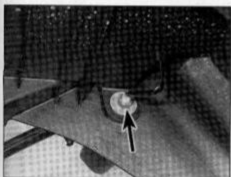
12.9 The rear turn signal assembly is secured to the mudguard by a single nut (arrow)
