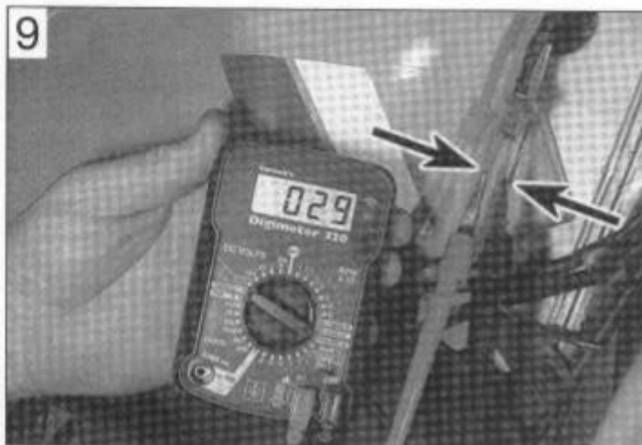
Continuity check of front brake light switch using a meter - note split pins used to access connector terminals
