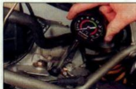
3.20 Using a rubber-cone type cylinder compression gauge
