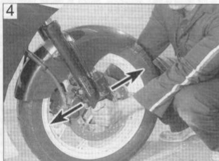
Checking the steering head bearings for freeplay
