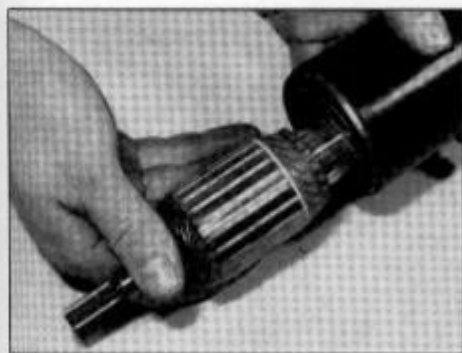
31.22a Slide the armature into the main housing ...
