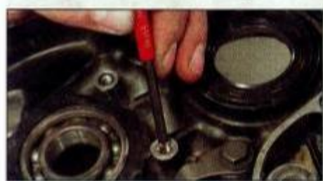
2.30 ... break off the tang when complete
