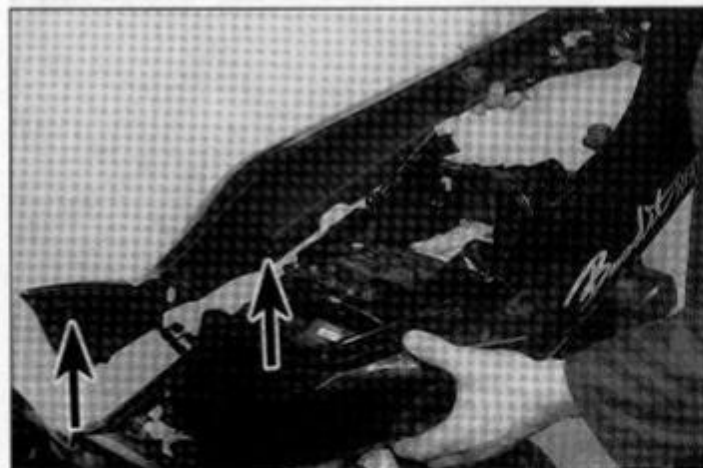
4.3d Carefully release the pegs (arrows) then remove the side panel assembly
