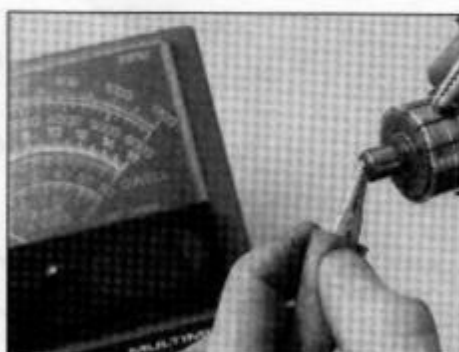
31.9b There should be no continuity between the commutator bars and the armature shaft
