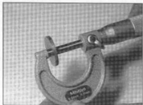
Tappet shims are measured with a micrometer
