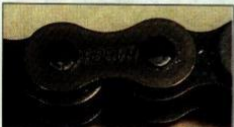
8.10 Typical chain size and type marking
