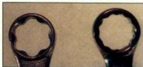
2.21 Comparison of surface drive ring spanner (left) with 12-point type (right)
