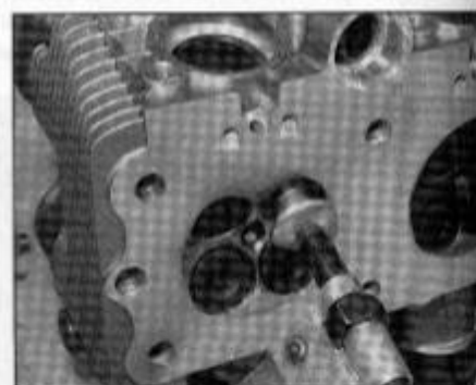
14.6b . . . and the valve. The compressor must only contact the valve and not the soft aluminium of the head - use a spacer if the plate on the compressor is too big for the valve
