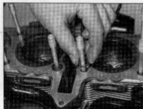
12.14 Fit new O-rings around the two front centre studs and all four end studs
