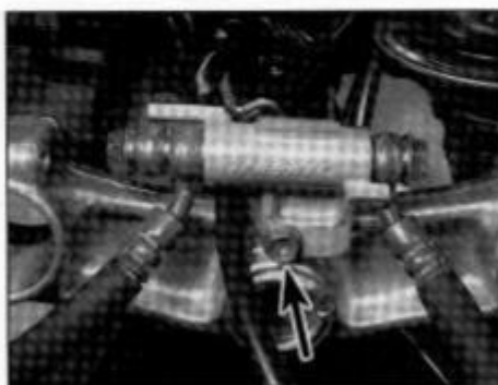
8.5a Remove the bolt securing the brake hose union (arrow) . . .
