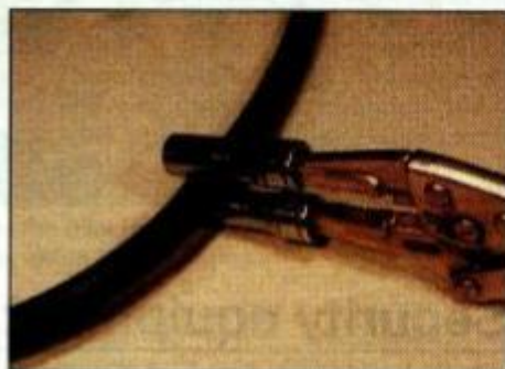
9.3 ... two sockets and a pair of self-locking grips ...
