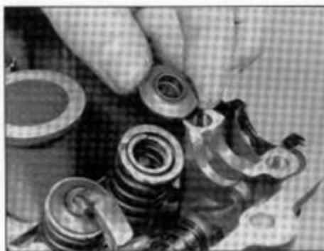
14.29d Make sure the spring retainer is the correct way round
