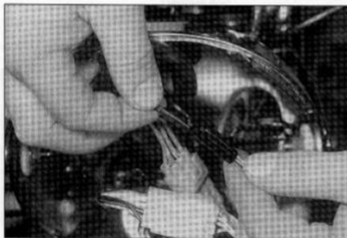
12.2 The front turn signal wire connectors are inside the headlight
