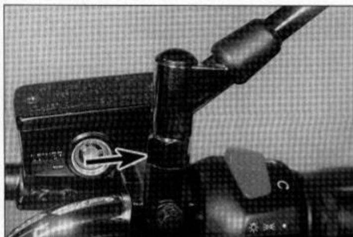
2.1 Unscrew the mirror using a spanner on the nut (arrow)
