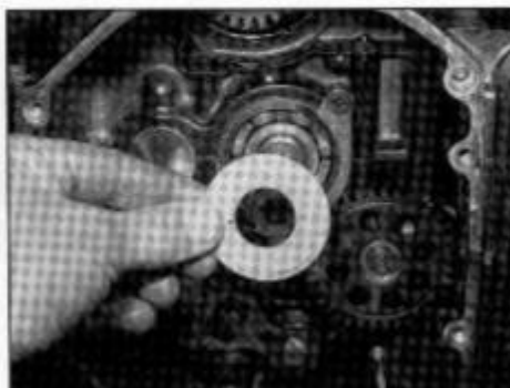
18.45 Fit the inner thrust washer with its flat side facing out
