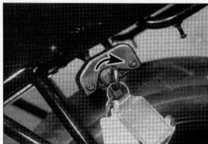
3.1 Turn the key clockwise to unlock the seat
