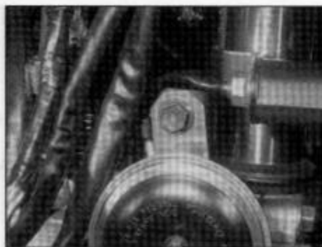
28.5 Each horn is secured by a single bolt
