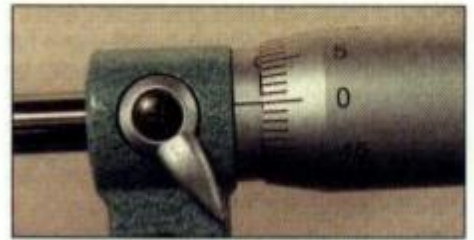
3.2 Check micrometer calibration before use
