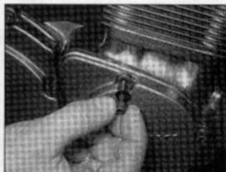
4.16b A sealing washer is fitted on the top bolt
