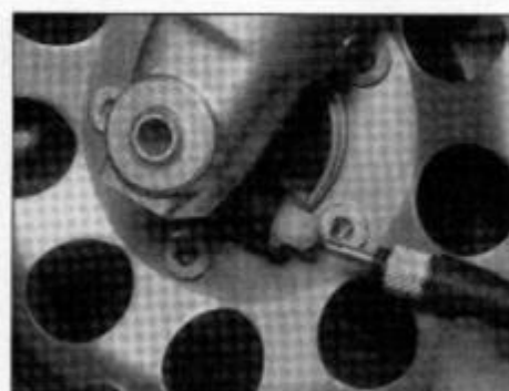
14.16 Align the notch in the cable end with the drive tab
