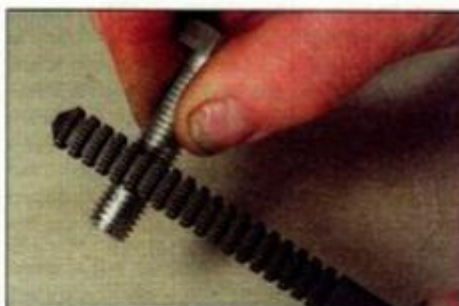
2.24 Using a thread restorer file
