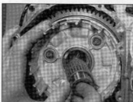
18.33b ... then slide the spacer and needle bearing into the centre of the housing
