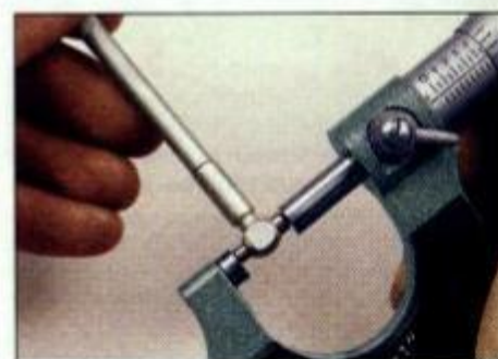
3.8 ... then measure the gauge with a micrometer
