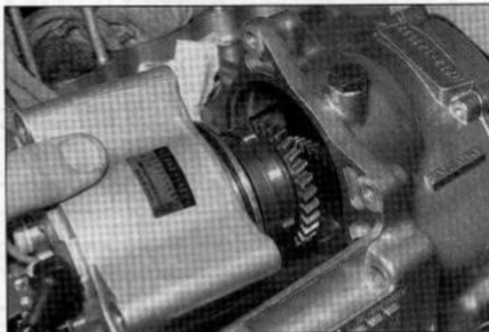
34.18 ... and install the alternator
