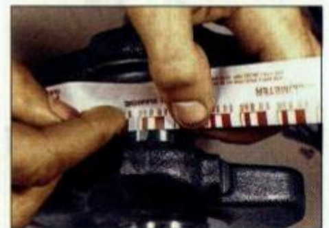
3.16 Measuring the width of the crushed Plastigauge
