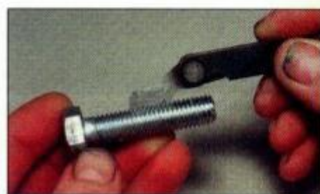
2.12 Using a thread gauge to measure pitch
