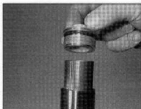
7.27 Fit a new O-ring onto the top bolt and thread the bolt into the fork tube
