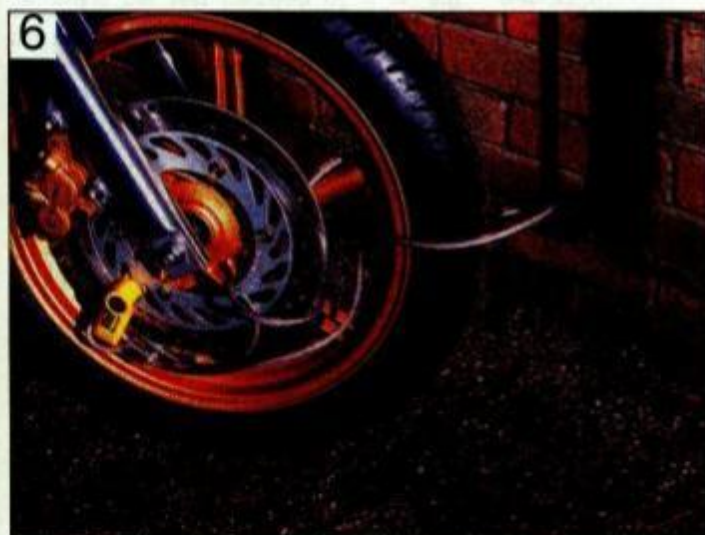
A disc lock combined with a security cable provides additional protection
