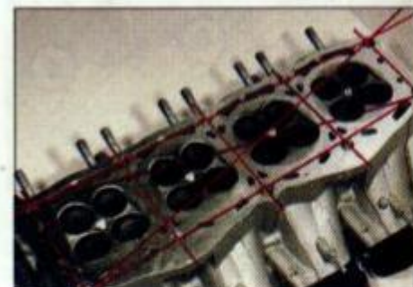
3.23 Check for warpage in these directions
