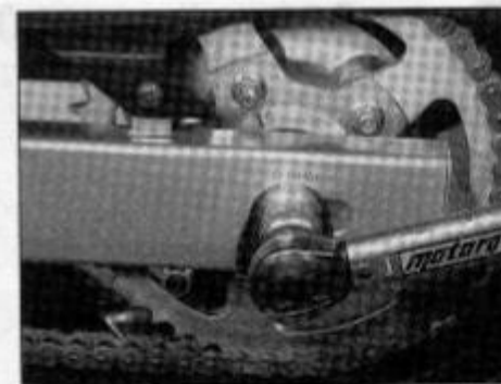
2.9 Tighten the axle nut to the specified torque setting
