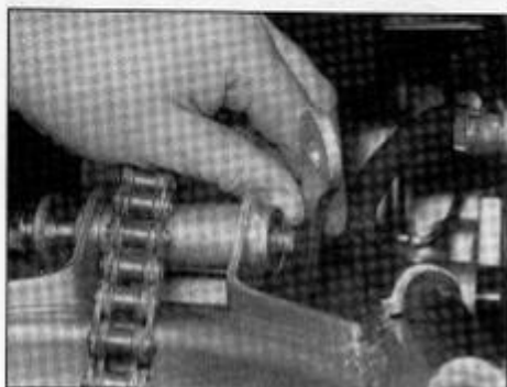
11.5b ... and remove the right-hand rod
