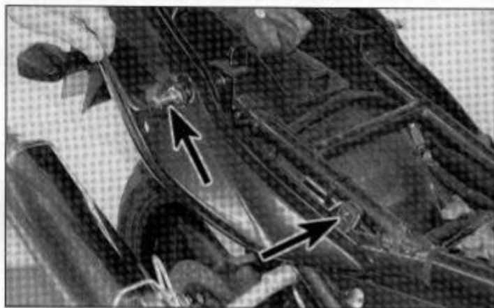
4.8a Remove the side panel fixing screws ...
