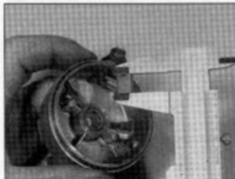
31.7 Measure the length of each brush
