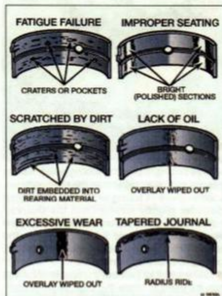
5.17 Typical bearing failures
