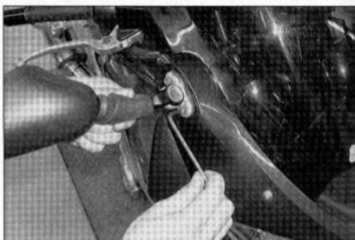
2.3 Unscrew the two bolts securing the rear view mirrors
