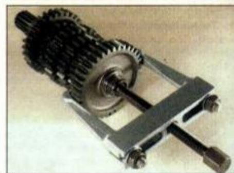
5.4 Where no access is available to the rear of the bearing, it is sometimes possible to draw off the adjacent component
