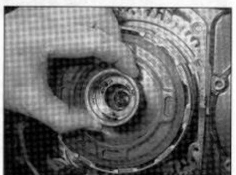
18.50a Fit the diaphragm spring holder into the pressure plate ...
