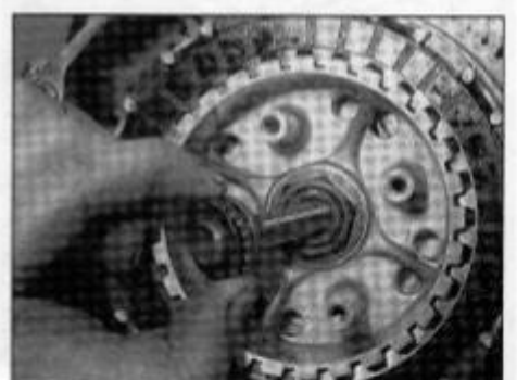
18.3c Withdraw the pushrod end piece along with the thrust washer and release bearing
