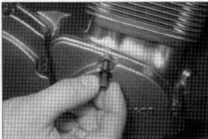
18.11 A sealing washer is fitted on the top bolt
