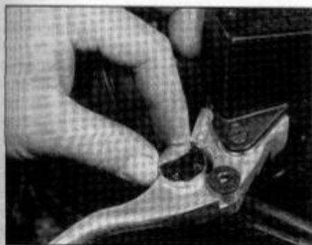
14.7 Adjusting the front brake lever span
