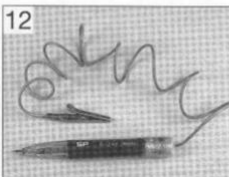
A simple test light can be used for voltage checks
