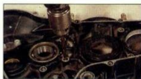
2.26 To install a thread insert, first drill out the original thread ...
