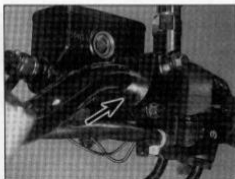
5.21a Align the mating surfaces of the clamp with the punch mark (arrow) ...
