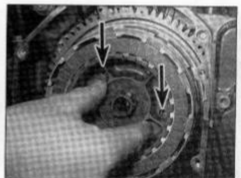
18.18 Grasp the clutch centre and pull it off with the plates. Two M6 bolts can be threaded into the holes (arrows) to aid removal
