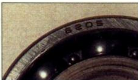
5.16 Typical bearing marking
