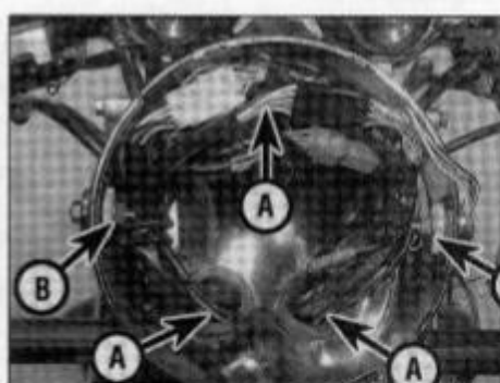
8.3b Feed the wiring through the holes (A), then unscrew the nuts (B) and remove the bolts
