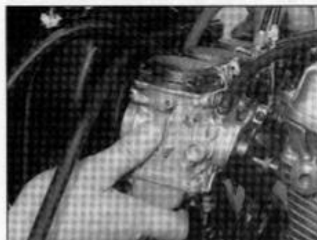
6.8b ... and ease them out of the adapters
