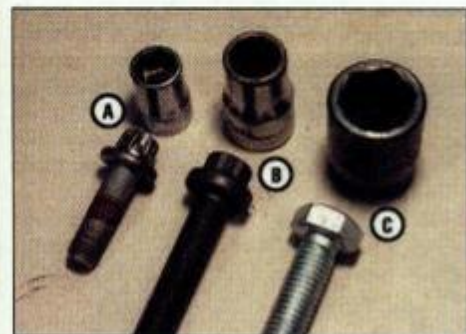
2.2 External Torx (A), splined (B) and hexagon (C) fasteners, with corresponding sockets
