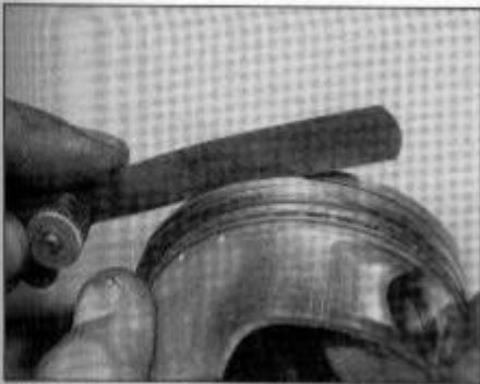
16.11 Measure the piston ring-to-groove clearance with a feeler gauge
