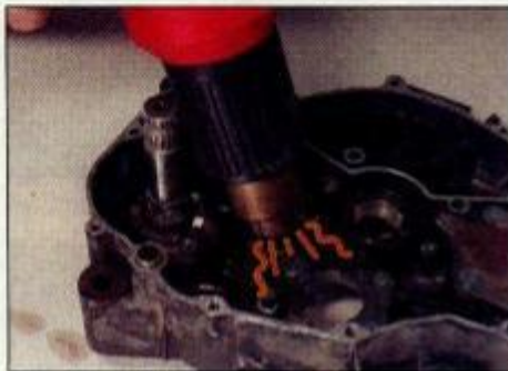
2.15 Using heat to free a seized fastener
