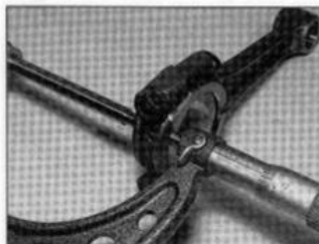
31.7a Measure the width of the connecting rod ...
