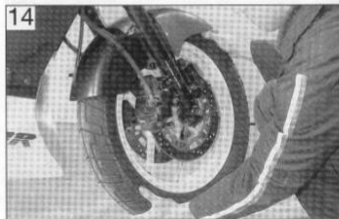
Check for wheel bearing play by trying to move the wheel about the axle (spindle)
