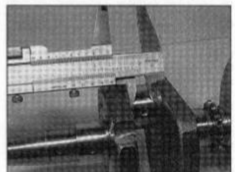
31.7b ... and of the corresponding crankpin
