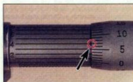
3.6 ... and 0.004 mm on vernier scale
