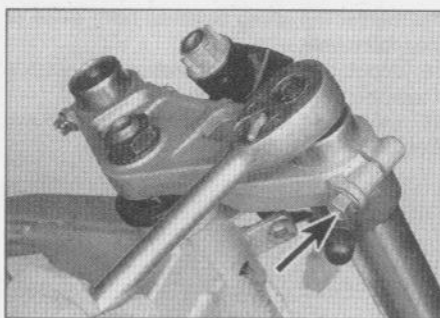
7.11 If the forks are going to be disassembled, loosen the upper clamp bolt, then loosen the top plug with a 1/2 inch drive ratchet
