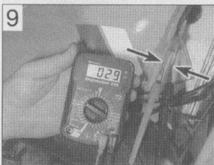
Continuity check of front brake light switch using a meter - note split pins used to access connector terminals
