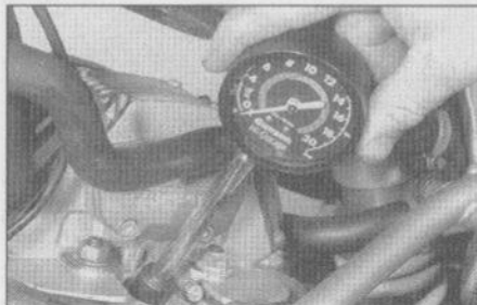
3.20 Using a rubber-cone type cylinder compression gauge
