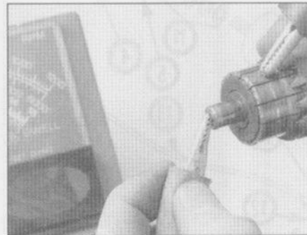
28.11b There should be no continuity between the commutator bars and the armature shaft
