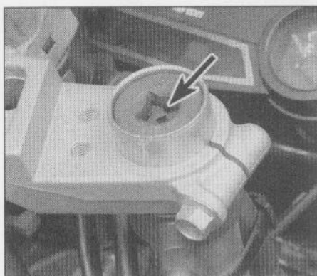
28.4 After the handlebar is removed and the fork upper pinch bolts have been loosened, the top plug can be removed
