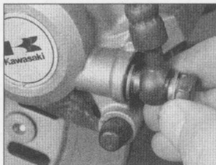
2.3a Unscrew the banjo fitting bolt, ...
