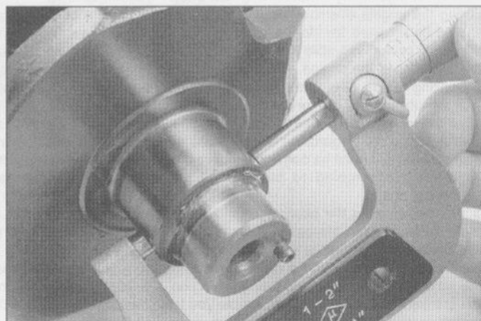
25.13 Measure the diameter of each crankshaft journal at several points to detect taper and out-of-round conditions
