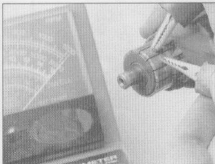
28.11a Continuity should exist between the commutator bars
