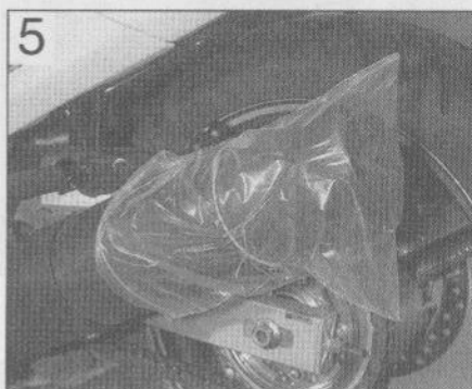
Exhausts can be sealed off with a plastic bag
