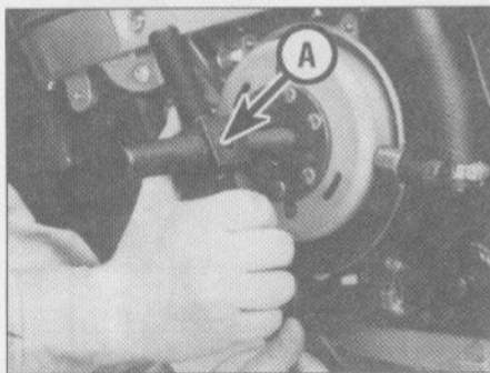
32.5 A special tool (A) is needed to pull the alternator rotor off - the rotor must be held stationary while doing this
