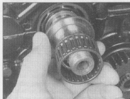
19.8b Remove the collar, bearing and spacer from the mainshaft
