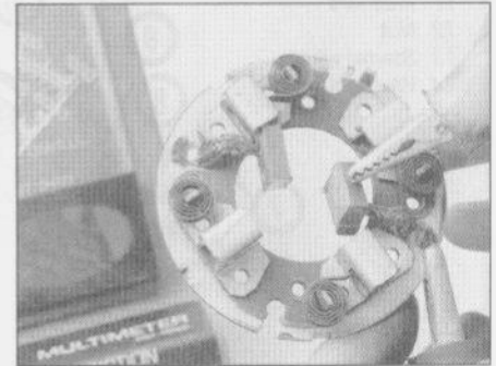
28.12 There should be almost no resistance (0 ohms) between the brushes and the brush plate
