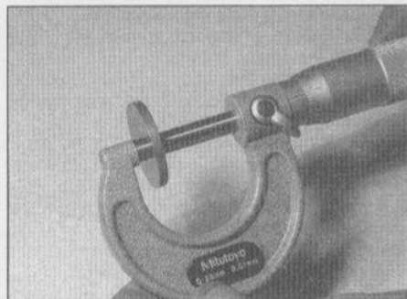
Tappet shims are measured with a micrometer
