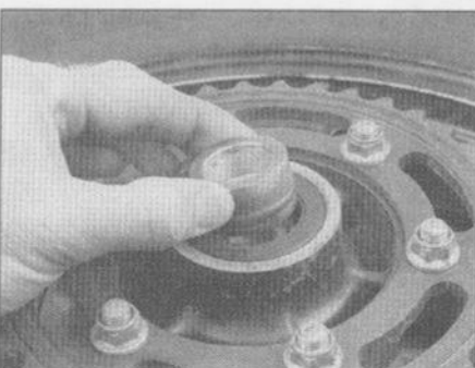
13.4a If you're removing the rear wheel bearings, lift out the coupling sleeve, . . .
