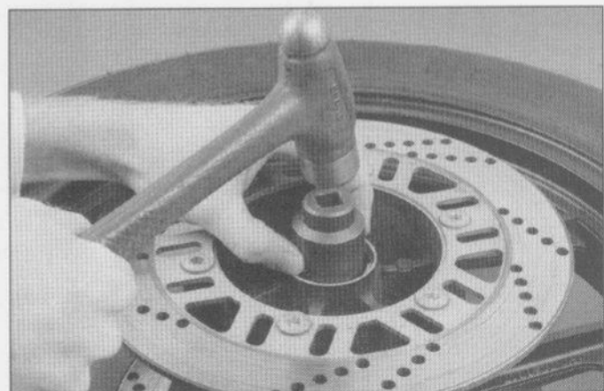
13.11 A socket of the appropriate diameter can be used to drive the bearing into the hub
