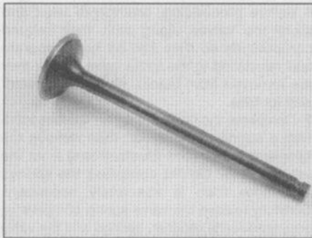
12.17 Check the valve face, stem and keeper groove for signs of wear and damage
