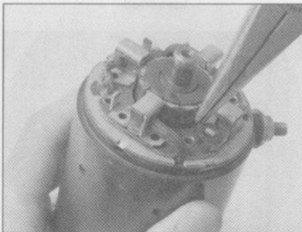
28.17b . . . then pull the end of the spring 1/2 turn clockwise and seat the end of it in the groove in the end of the brush
