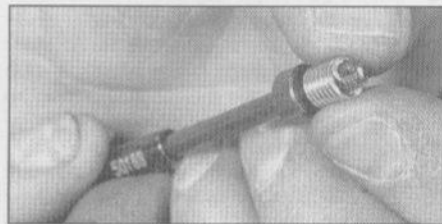
2.28 ... fit insert on the installing tool ...
