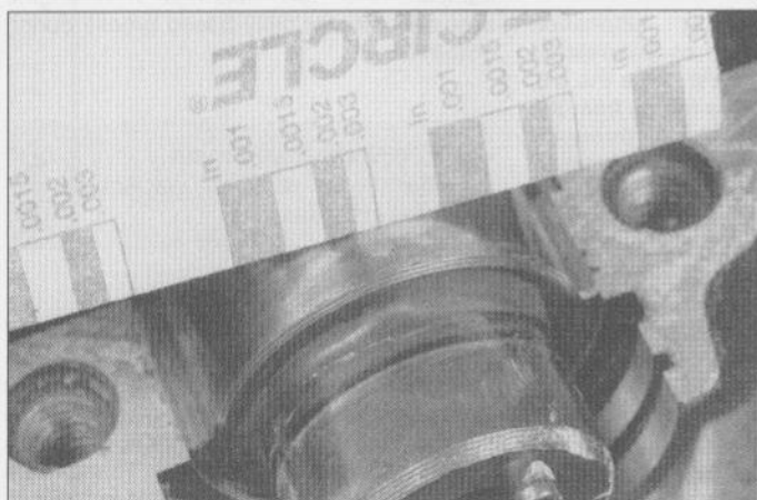
25.10 Measuring the width of the crushed Plastigauge (be sure to use the correct scale – standard and metric are included)
