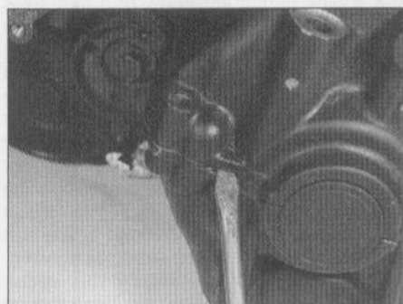
22.10a There's a pry point at each end of the crankcase...
