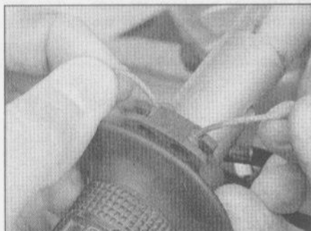
9.7 Align the cables with the slots in the throttle grip pulley, then slide the cable ends out
