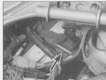
13.3 Location of the turn signal flasher (arrow)
