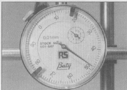
3.17 Dial gauge reading of 1.48 mm
