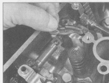
9.18a Lift the rocker arms out of the shafts . . .
