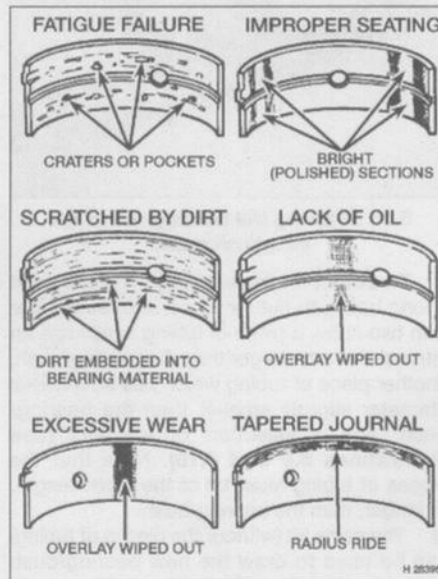
5.17 Typical bearing failures
