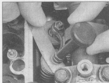
20.8 Checking the valve clearance
