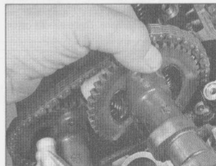
9.6a Lift the camshaft chain, disengage it from the sprocket and guide the camshaft out
