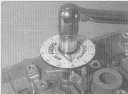
Angle-tightening cylinder head bolts
