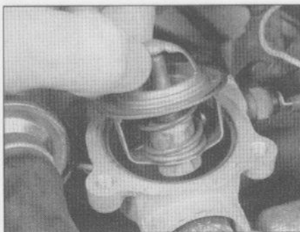
6.4b Remove the thermostat from the housing, noting how it is installed
