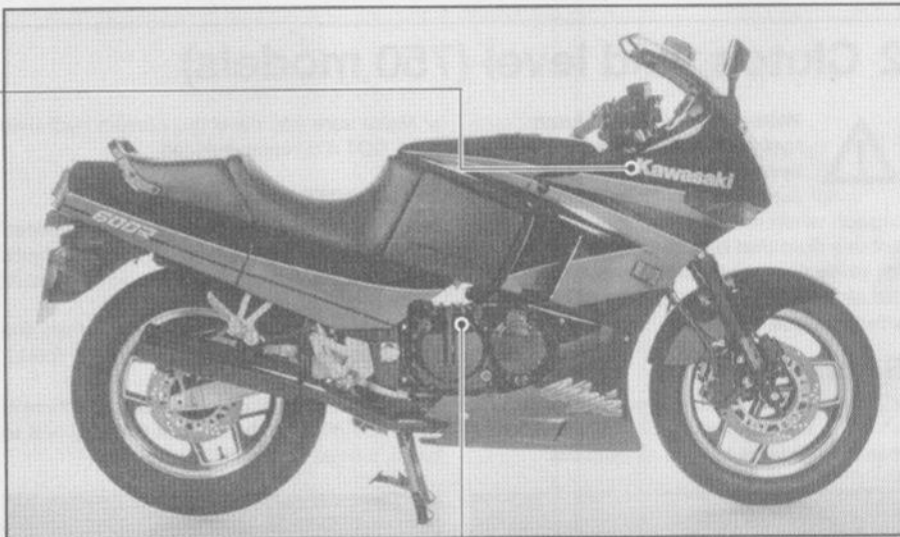
The engine number (arrow) is stamped into the top of the crankcase, just inboard of the clutch cover
