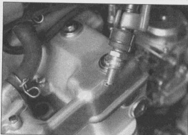
2.3 With the wire attached, ground (earth) a spark plug to the engine and operate the starter - bright blue sparks should be visible
