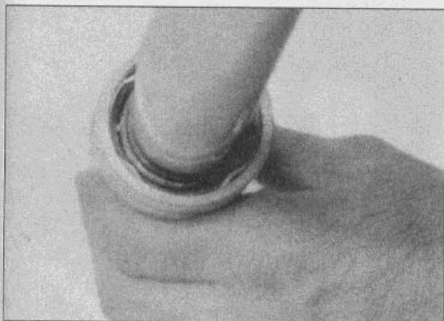
4.21 Install the retaining ring and make sure it seats in its groove
