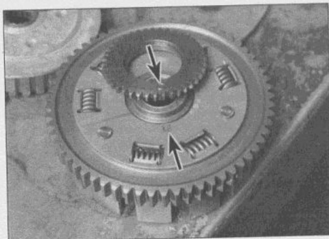
25.30a The pin in the oil pump drive gear must engage the notch in the clutch housing (arrows). . .
