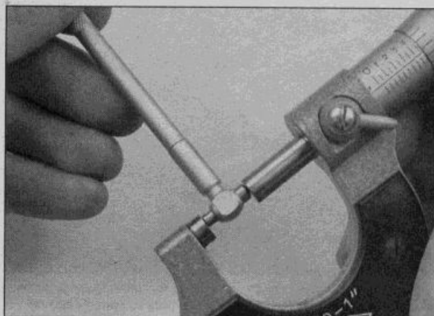
9.34c . . .and a micrometer is used to measure the gauge
