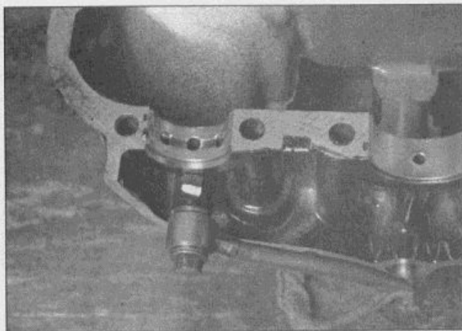
27.5a The balancer bearing inserts near the external oil line have oil grooves. . .
