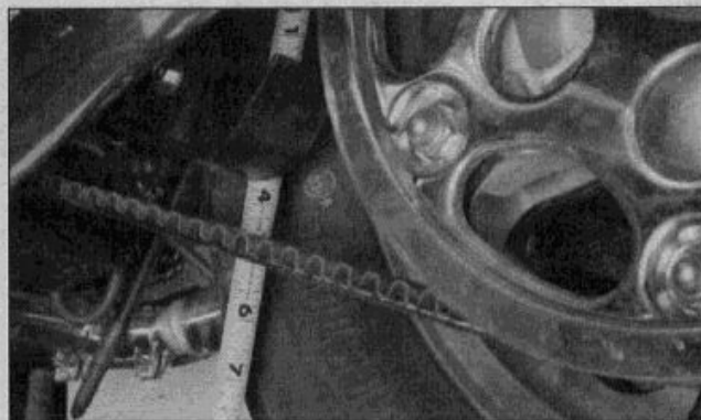
11.3 Push up on the bottom run of the belt and measure how far it deflects - if it's not within the specified limits, adjust the slack in the belt
