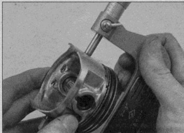
14.14a Measure the piston diameter with a micrometer
