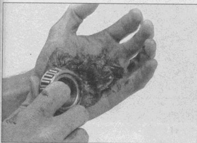
5.19 Work the grease completely into the rollers
