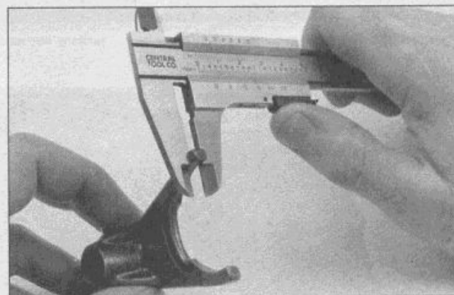
31.7 Measure the thickness of the shift fork ears
