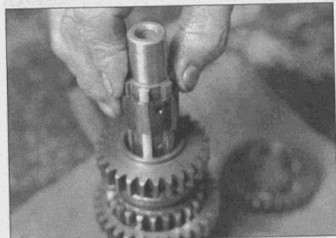
30.17g . . .and its bushing (align BOTH oil holes in the bushing with those in the shaft)
