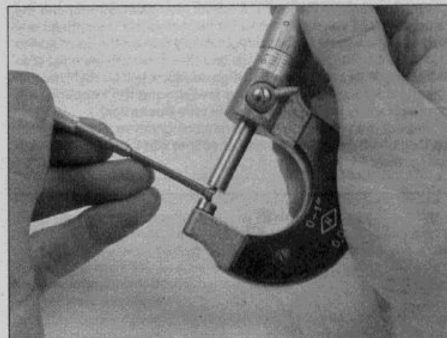
12.16b Measure the small hole gauge with a micrometer
