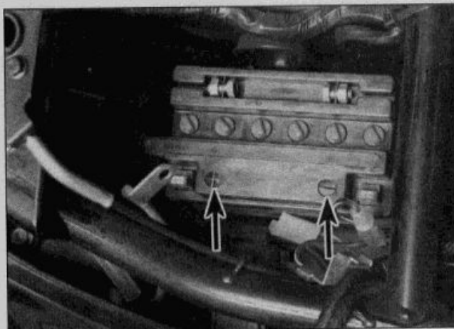
4.4 The positive terminal is identified by a plus mark molded into the top of the battery and the negative terminal is identified by a minus mark (arrows); ALWAYS disconnect the negative cable first and connect it last to prevent sparks which could cause a battery explosion
