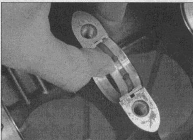
25.7 To remove a main bearing insert, push it sideways and lift it out
