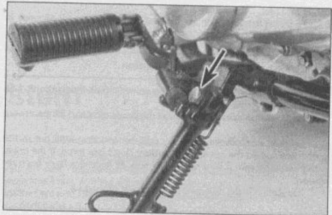
4.3 With the motorcycle securely supported, unhook the spring and remove the pivot bolt (arrow) to detach the sidestand
