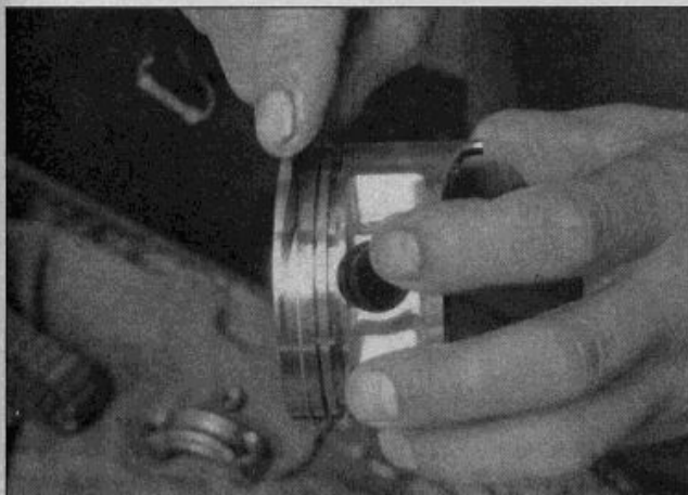
14.13 Measure the piston ring-to-groove clearance with a feeler gauge
