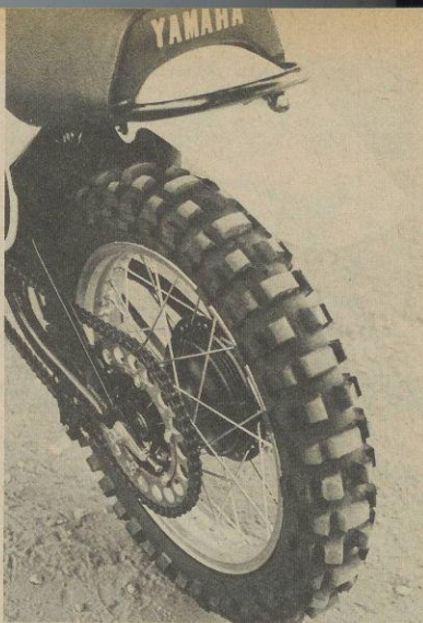
The sight of no shocks isn't the thrill it once was. The top arms of the swing arm push and pull on the shock beneath the tank.
