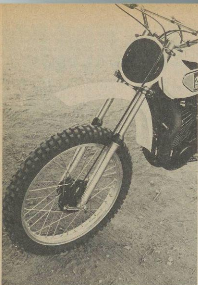
The one weak point on a fine racer: forks that are too soft and too flexible to cope with the weight transfer from the rear.
