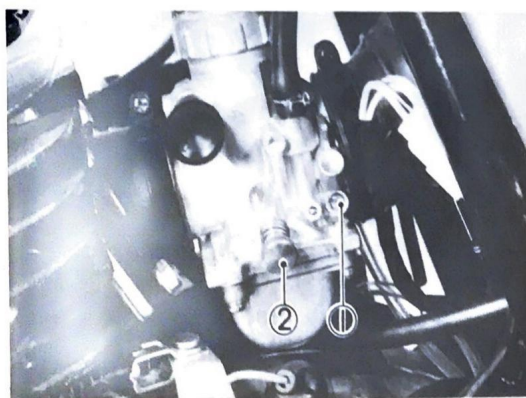
1. Pilot stop screw 2. Throttle stop screw
