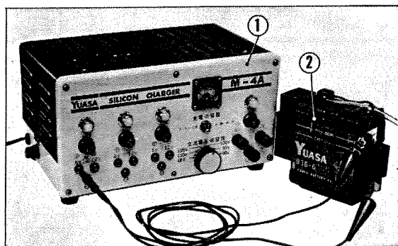
Fig. 5-18A. ① Charger ② Battery
