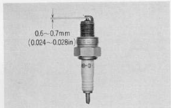
Fig. 5.10 Measuring spark gap
