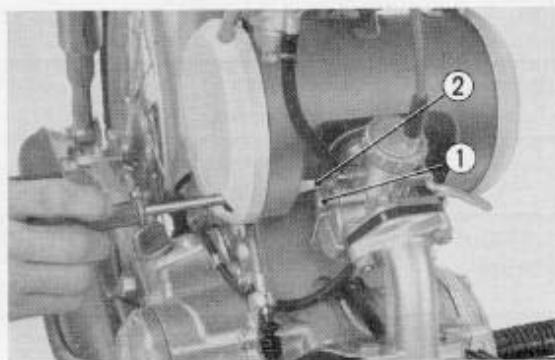
Fig. 6.2 Adjusting the idling (S 90) ① Throttle stop screw ② Air screw
