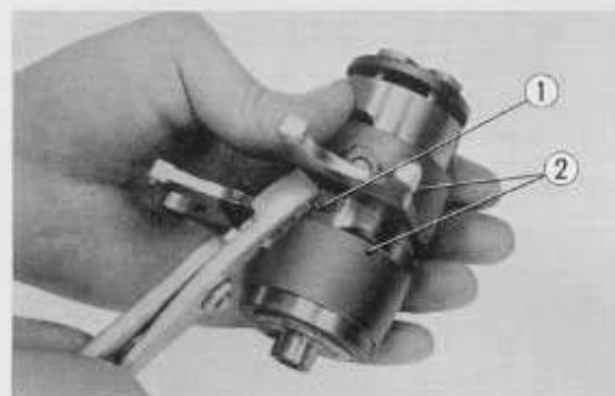
Fig. 3.98 Removing the gear shift fork
