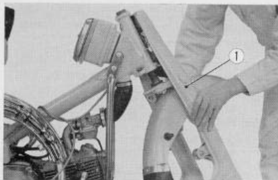
Fig. 4.36 Removing front fork ① Front fork
