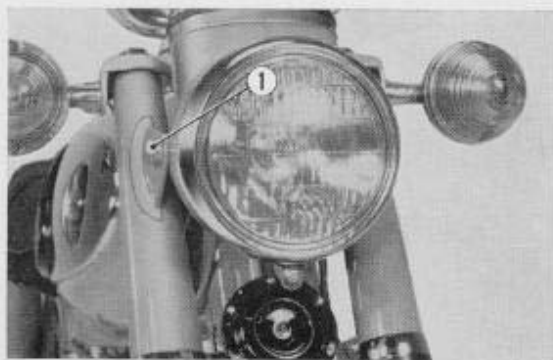
Fig. 4.25 Removing headlight ① 8×22 hex bolt
