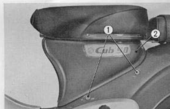
Fig. 4.45 Removing fuel tank ① Fuel tank mounting bolt ② Fuel tank
