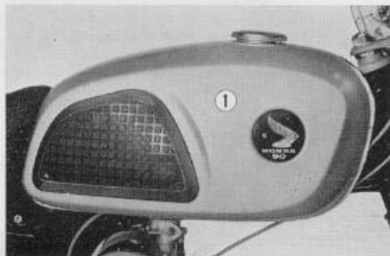
Fig. 4.39 B Fuel tank (CL 90) ① Fuel tank
