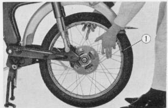
Fig. 4.95 Removing rear wheel ① Rear wheel.
