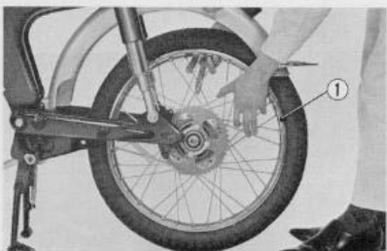
Fig. 4.73 Removing rear wheel ① Rear wheel
