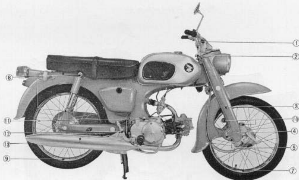
Fig. 5.42 Torquing points on right side
