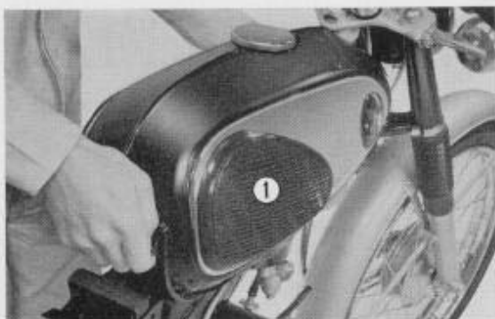
Fig. 4.42 Removing fuel tank ① Fuel tank
