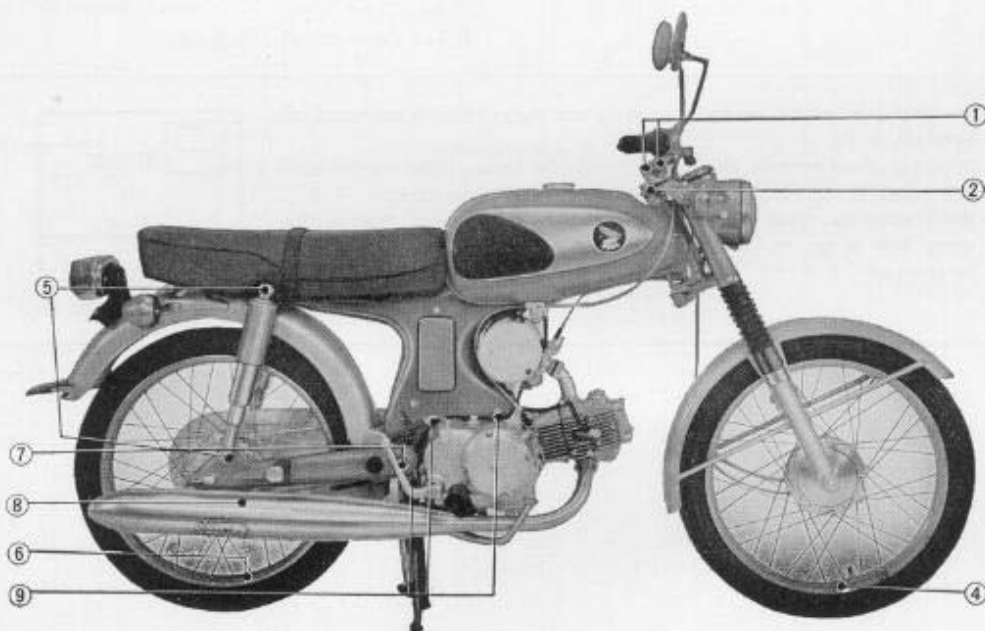
Fig. 5.40 Torquing points on right side
