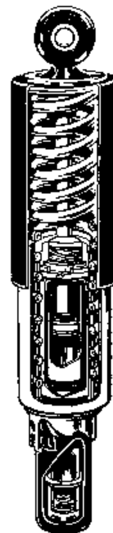
Illustration 12 "Ghost" view of Rear Suspension Unit
