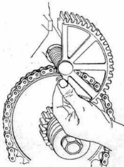
1. Hook free end of Spring over Top Spoke of Footstarter Quadrant.
