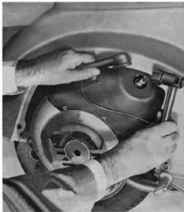
Fig. 10 - Dismantling spark - plug
