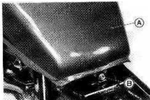
A. Fuel Tank
