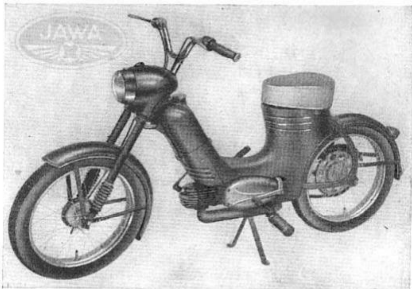
Above: The 50 c. c. ultra-lightweight Jawa motor-cycle, model 550. Specification of model 555: engine - single-cylinder, two-stroke, air-cooled. Bore 38 mm, stroke 44 mm, swept volume 49,8 c. c., compression ratio 7 : 1, power output 2,2 b. h. p. at 5500 r. p. m. Jikov 2914 carburetter, three speed gearbox, primary transmission and final drive by chain. Magneto-generator ignition, 6 V, 18 W generator output. Overall length 1780 mm (71 ins.), width across handlebar 560 mm (22 ins.), overall height 938 mm (37 ins.), weight 54 kg (119 lbs.). Top speed 60 km p. h. (38 m. p. h.), fuel consumption 1,8 litre per 100 km (157 m. p. g.). Maximum gradient climbed 22 per cent.
