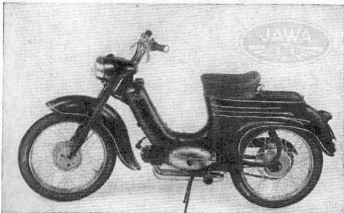
Above: The 50 c. c. ultra-lightweight Jawa motor-cycle, model 550. Specification of model 555: engine - single-cylinder, two-stroke, air-cooled. Bore 38 mm, stroke 44 mm, swept volume 49,8 c. c., compression ratio 7 : 1, power output 2,2 b. h. p. at 5500 r. p. m. Jikov 2914 carburetter, three speed gearbox, primary transmission and final drive by chain. Magneto-generator ignition, 6 V, 18 W generator output. Overall length 1780 mm (71 ins.), width across handlebar 560 mm (22 ins.), overall height 938 mm (37 ins.), weight 54 kg (119 lbs.). Top speed 60 km p. h. (38 m. p. h.), fuel consumption 1,8 litre per 100 km (157 m. p. g.). Maximum gradient climbed 22 per cent.
