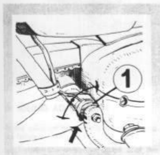
Fig. 5 - Adjustment of the stop-light switch
