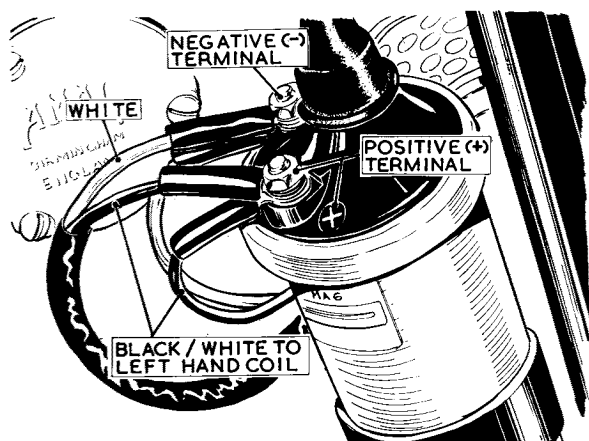
FIG. B.26. Coil connections.
