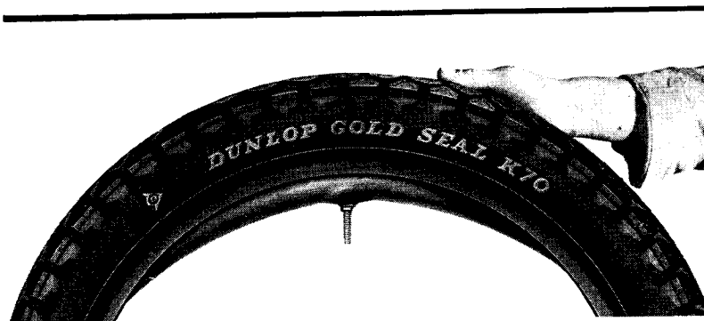
FIG. F.23. Cover and tube assembled ready for fitting.
