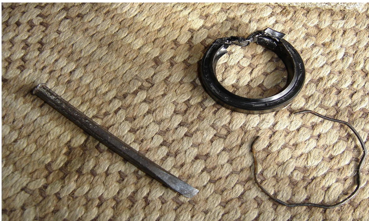
Close up of the chisel, seal retaining ring or “ring oil seal stopper” and the mangled fork seal.
