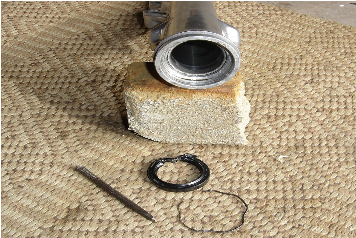
Close up of the chisel, seal retaining ring or “ring oil seal stopper” and the mangled fork seal.
