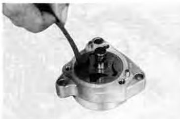
Checking tip clearance
