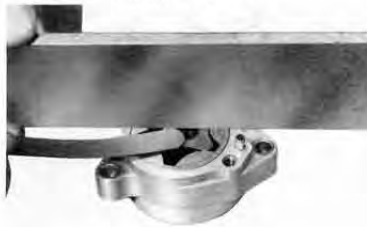
Checking side clearance
