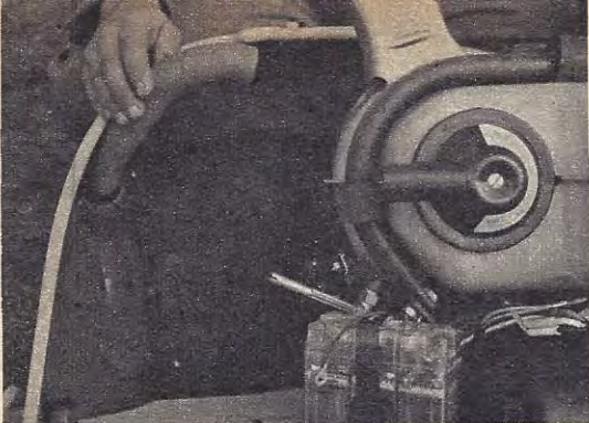
AIR FILTER is oil-soaked to trap dust entering engine. The flexible hose must be securely connected to the filter
