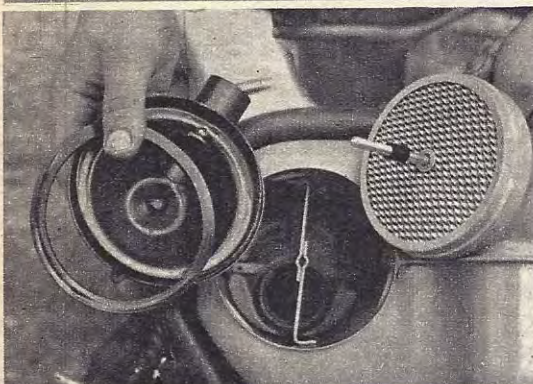
AIR FILTER removed from housing. Note rubber sealing ring. Filter must be fitted firmly to keep out all road dirt
