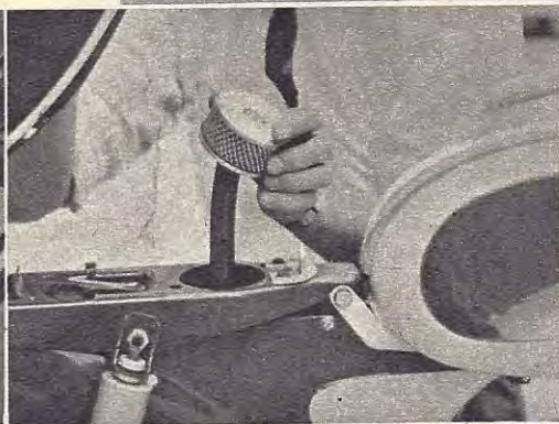
AIR-FILTER cartridge situated below the dual-seat should be impregnated with SAE 20 oil. Clean every 1,000 miles
