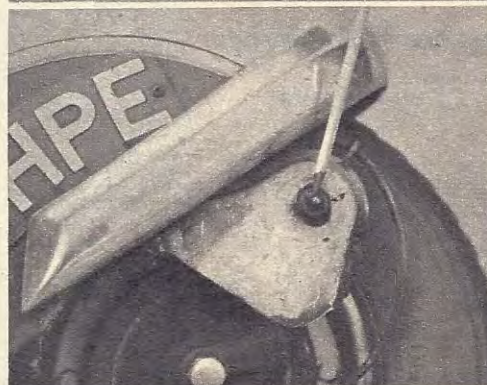
FRONT SUSPENSION should be greased at least every 1,000 miles or so, according to conditions, through this nipple
