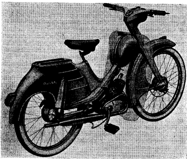
FIG. 4. THE QUICKLY-L This model extends the degree of fairing employed, has redesigned handlebars and sprung rear suspension.
