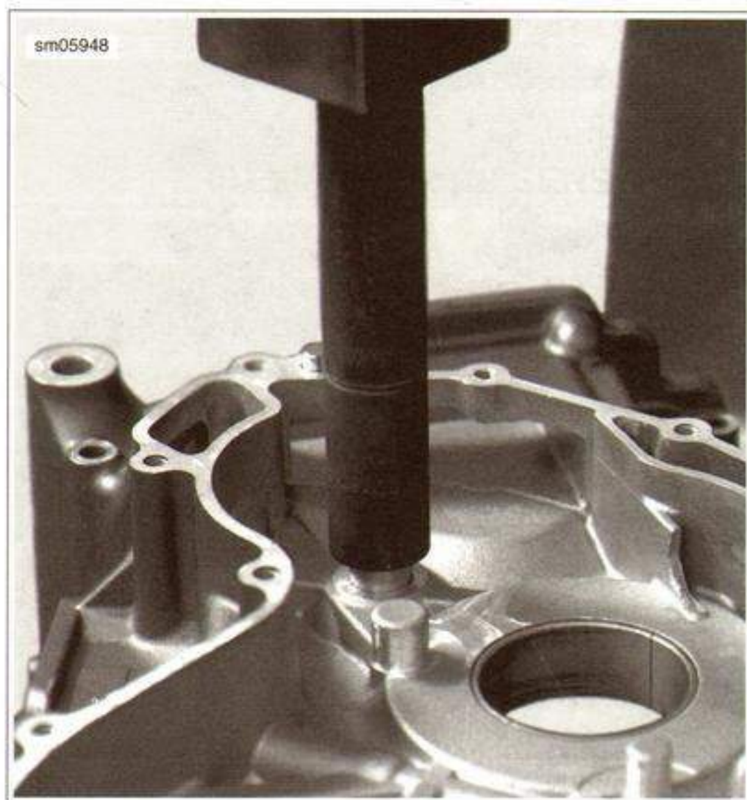
Figure 3-182. Water Pump Shaft Case Bearing Installer (B-49403)
