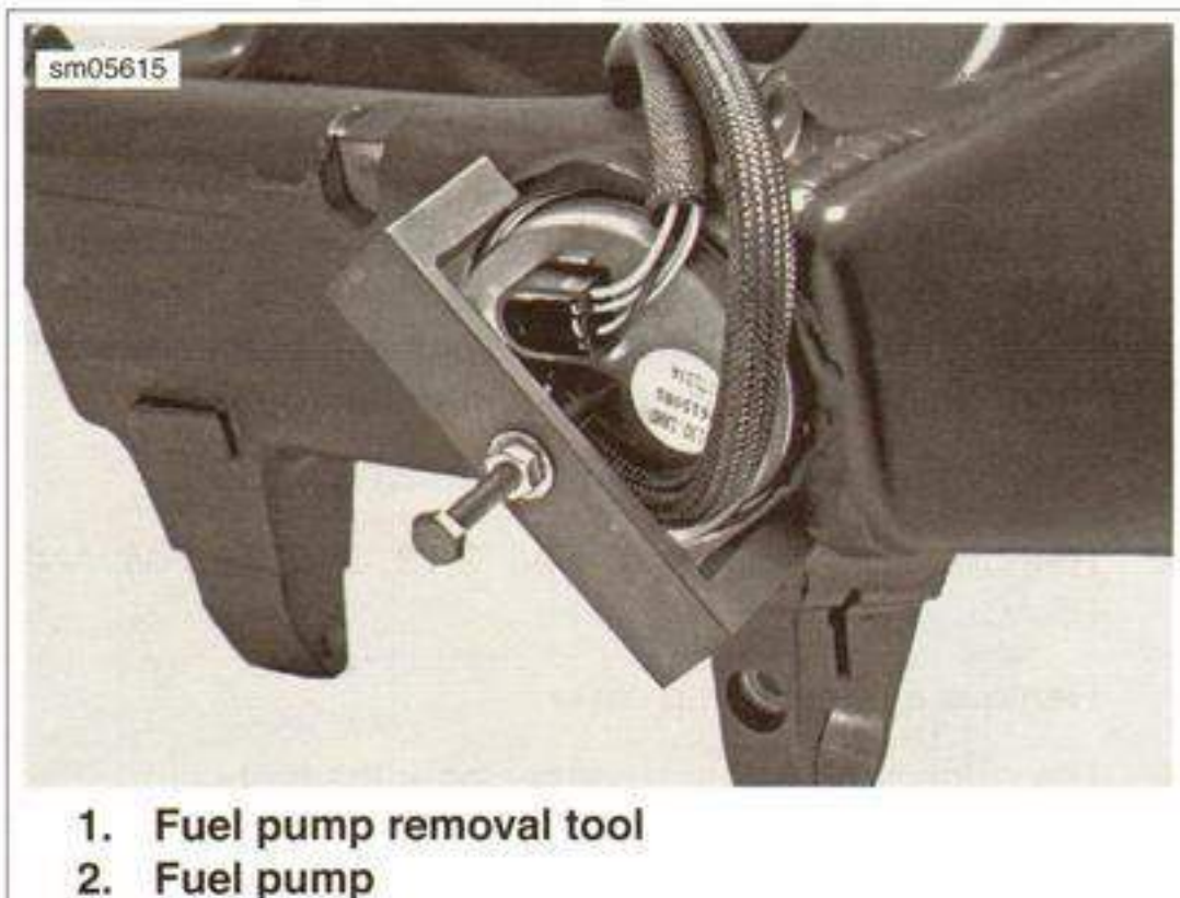
Figure 4-72. Fuel Pump Removal
