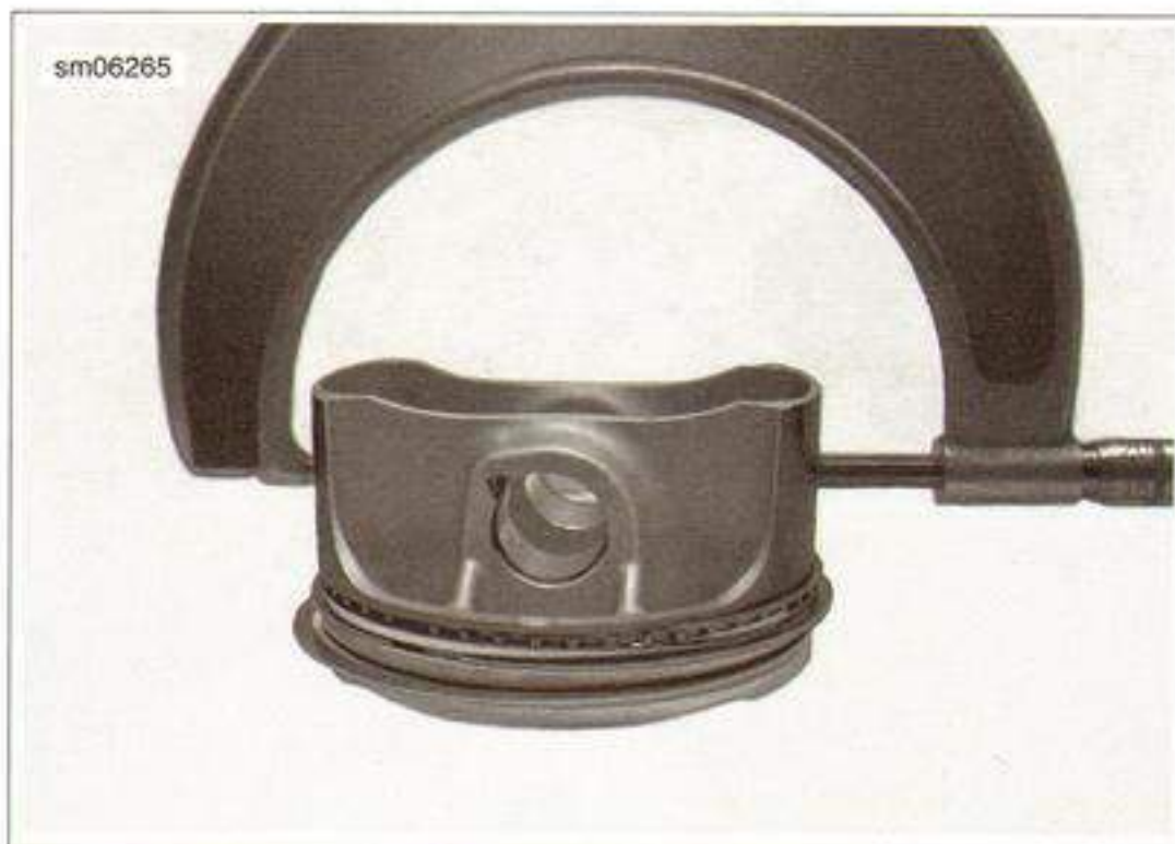
Figure 3-100. Measuring Piston Diameter
