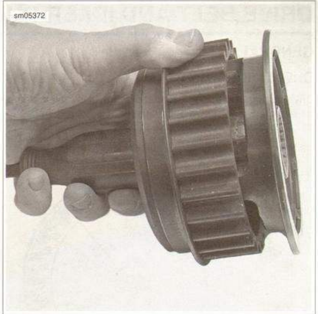
Figure 6-111. Separating the Pulley Assembly
