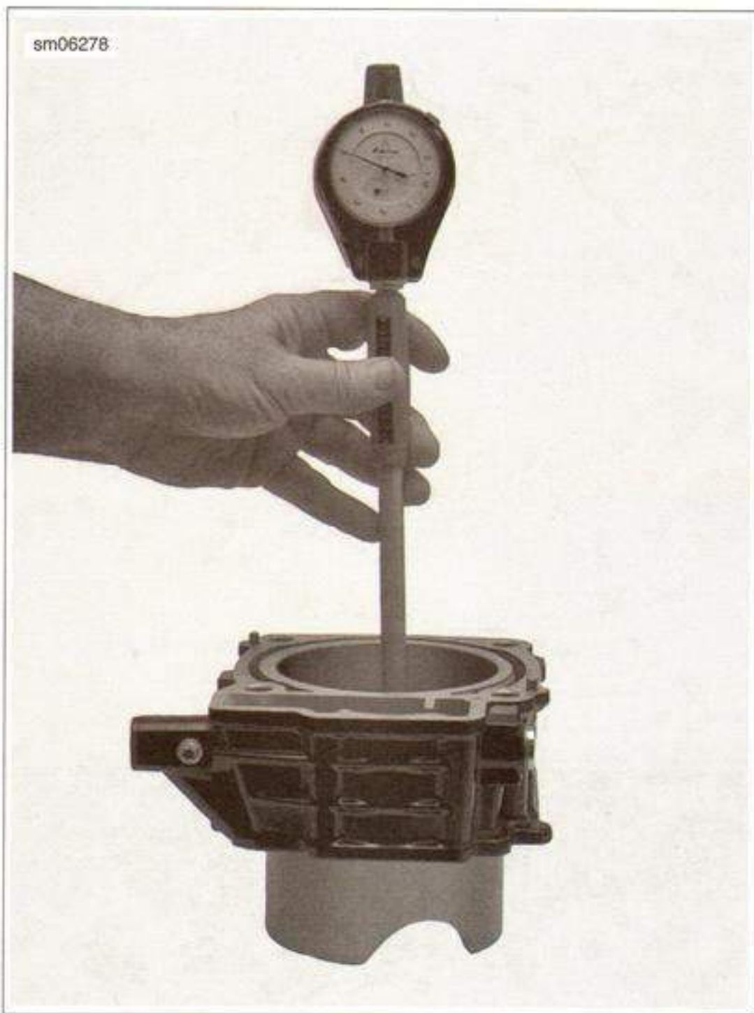
Figure 3-99. Measuring Cylinder Bore
