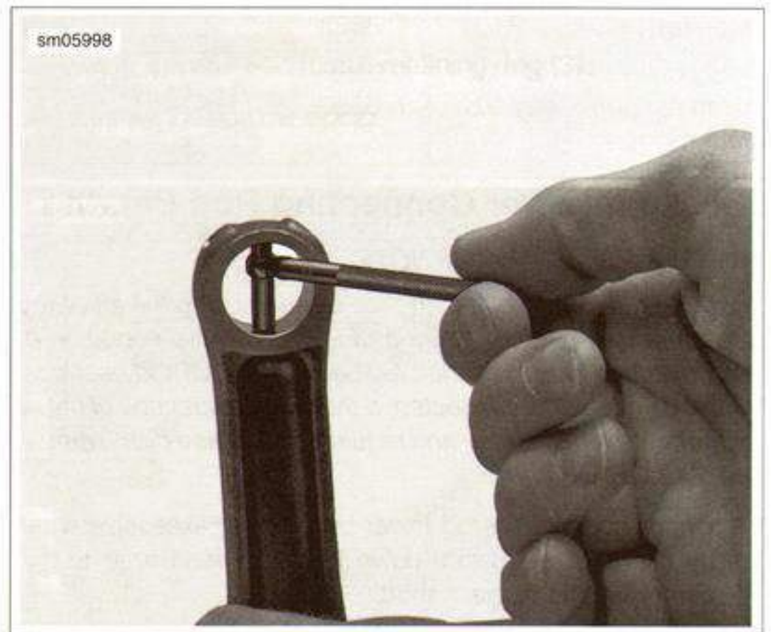
Figure 3-97. Connecting Rod Piston Pin Bore Measurement
