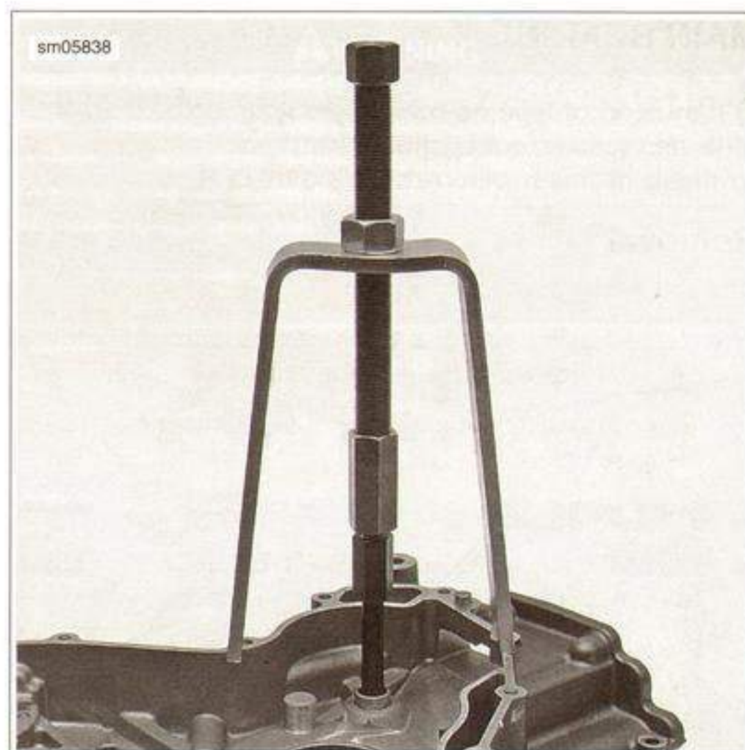
Figure 3-181. Remove the Water Pump Shaft Case Bearing
