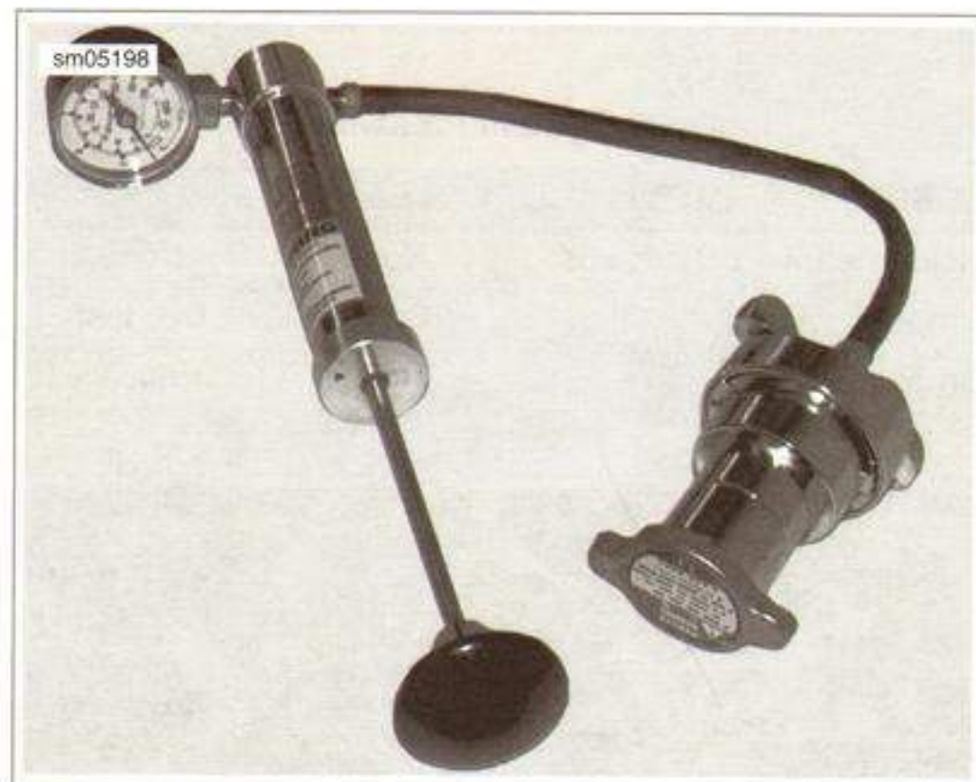
Figure 5-4. Pressure Cap Test
