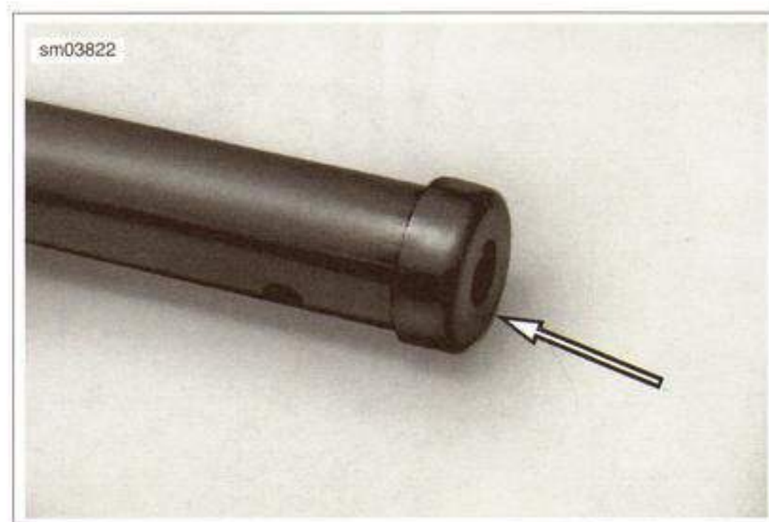
Figure 2-92. Centering Plate on Bottom of Damper Rod
