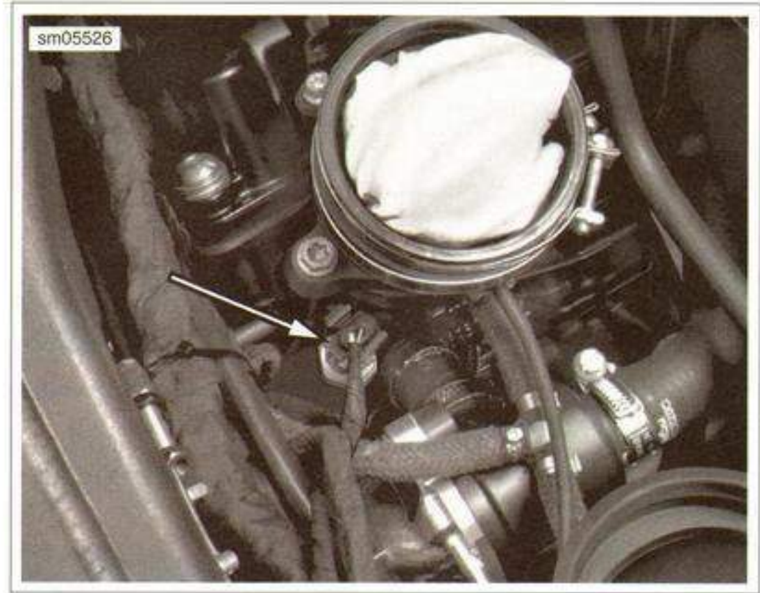
Figure 3-22. Engine Temperature Sensor
