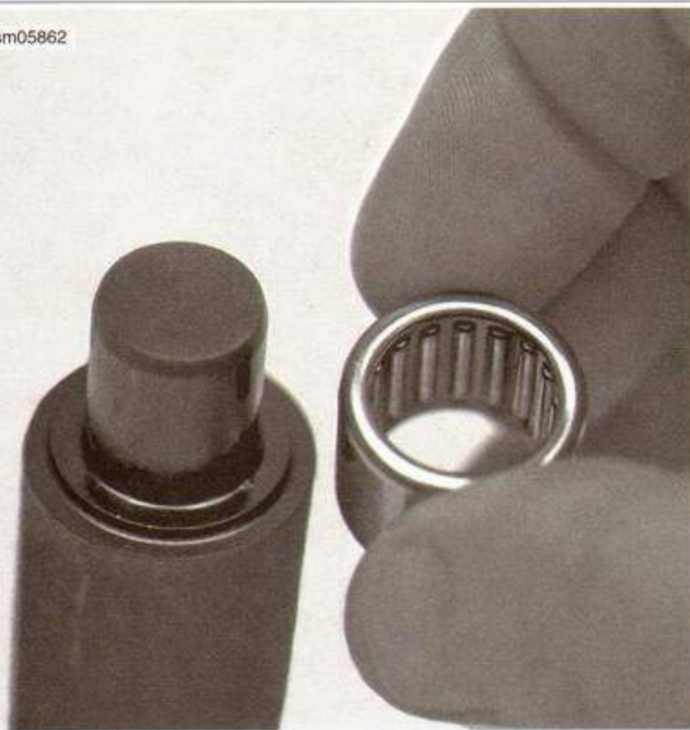
Figure 3-154. Top Balancer Needle Bearing Installer
