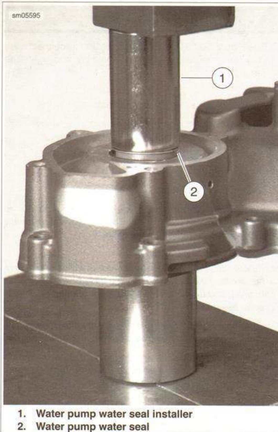
Figure 5-22. Installing Water Pump Water Seal
