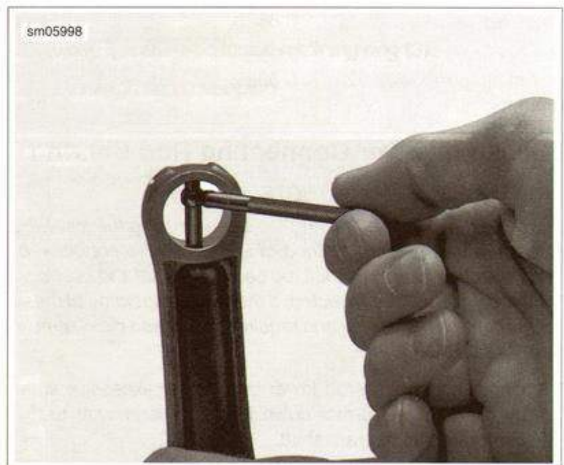
Figure 3-97. Connecting Rod Piston Pin Bore Measurement
