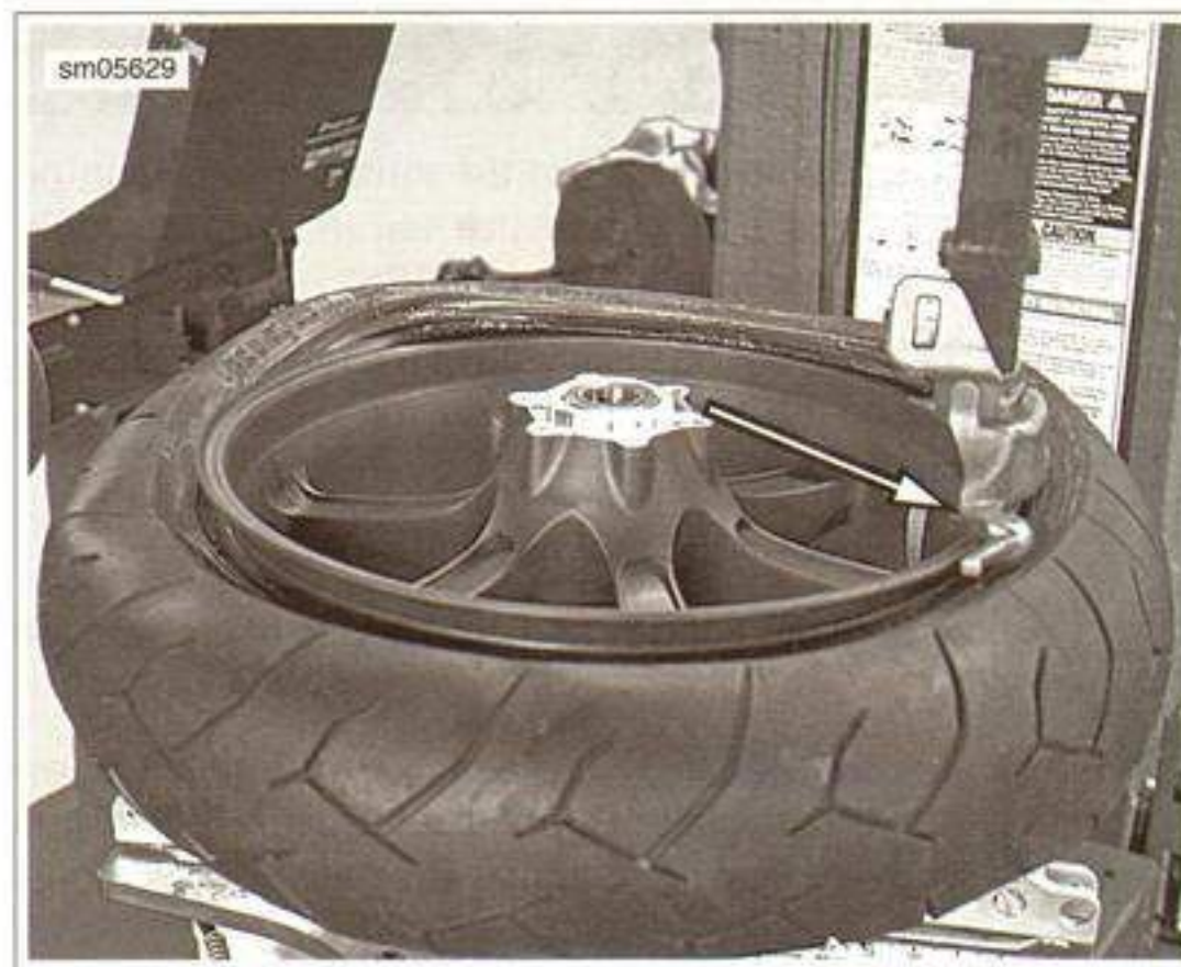
Figure 2-16. Feeding the Upper Bead onto the Rim
