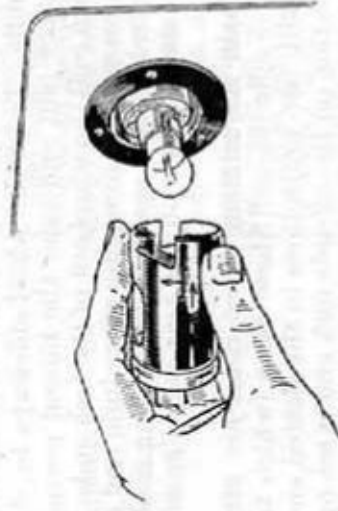
FIG. 80. LUCAS REAR LAMP (TYPE MT211) Fit the cover as indicated by the two arrows.
