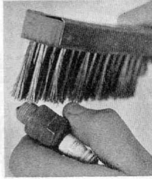
FIG. 37. BEFORE FITTING A PLUG, CLEAN ITS THREADS WITH A WIRE BRUSH (Champion Sparking Plug Co., Ltd.)
