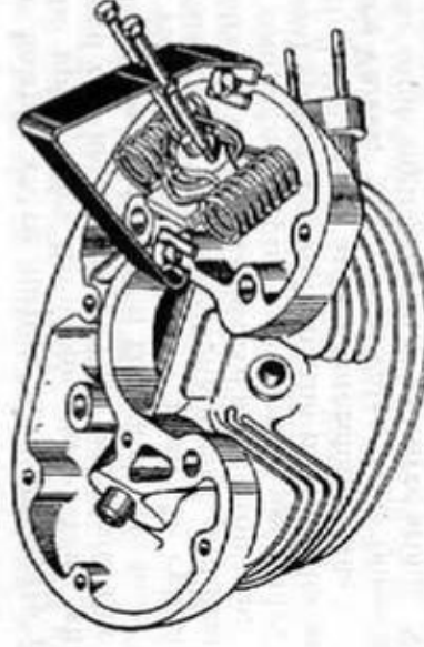
FIG. 77. MATCHLESS VALVE SPRING COMPRESSOR FITTED TO 1949 O.H.V. CYLINDER HEAD TO COMPRESS HAIRPIN VALVE SPRINGS
