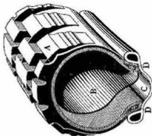
FIG. 8. SECTIONED MODERN TYRE (DUNLOP) AND RIM
