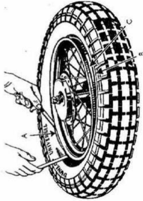
FIG. 13. CORRECT METHOD OF REMOVING A TYRE COVER
