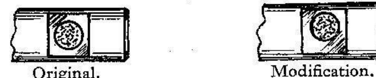
FIG. 28.—OIL-PUMP PLUNGER MODIFICATION FOR 1947-1948 MODELS.
