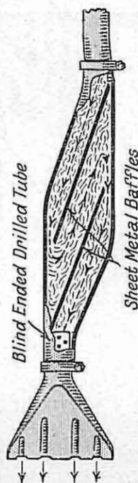
FIG. 6. DIAGRAM SHOWING PRINCIPLE OF MATCHLESS SILENCER
