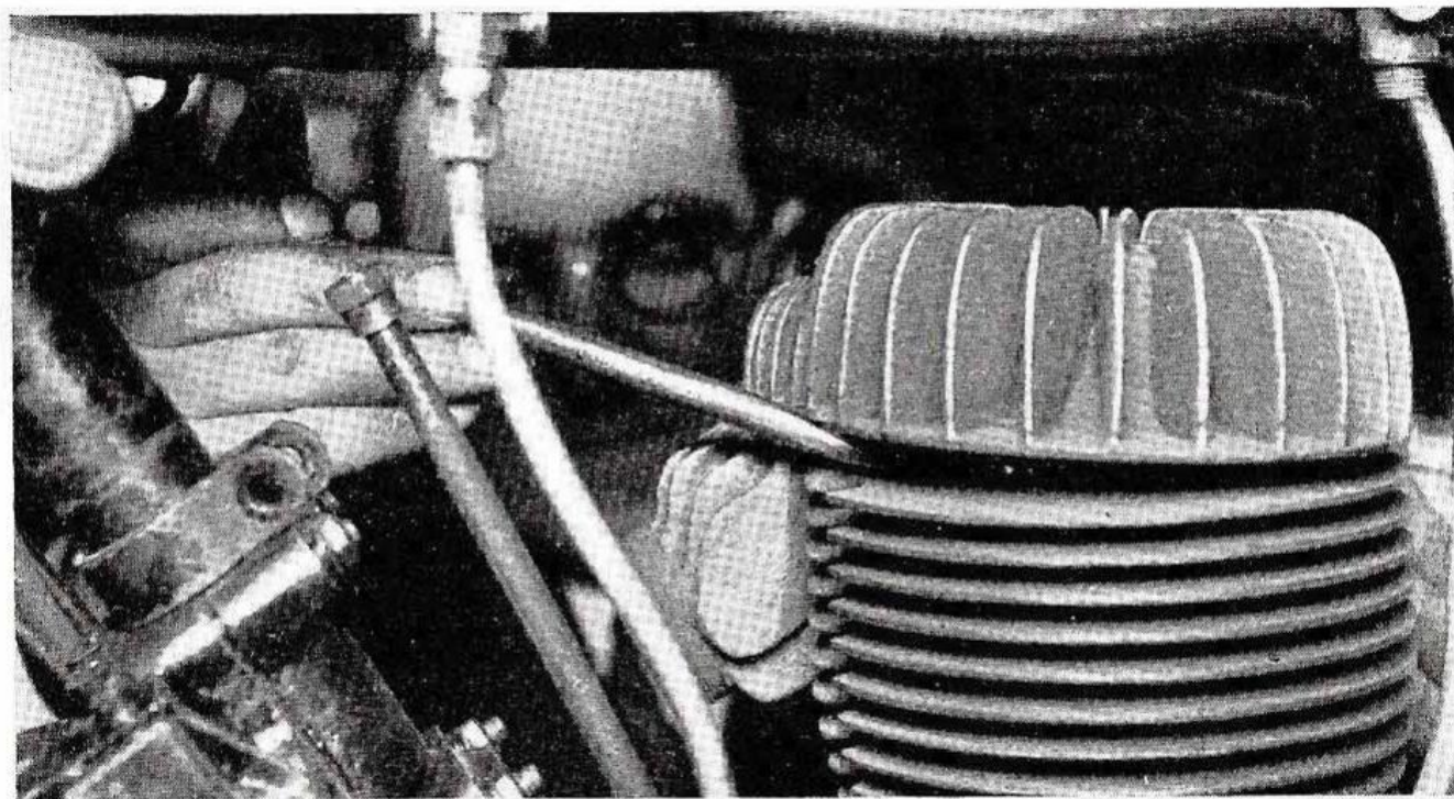
Fig. 3. —METHOD OF REMOVING CYLINDER HEAD.
