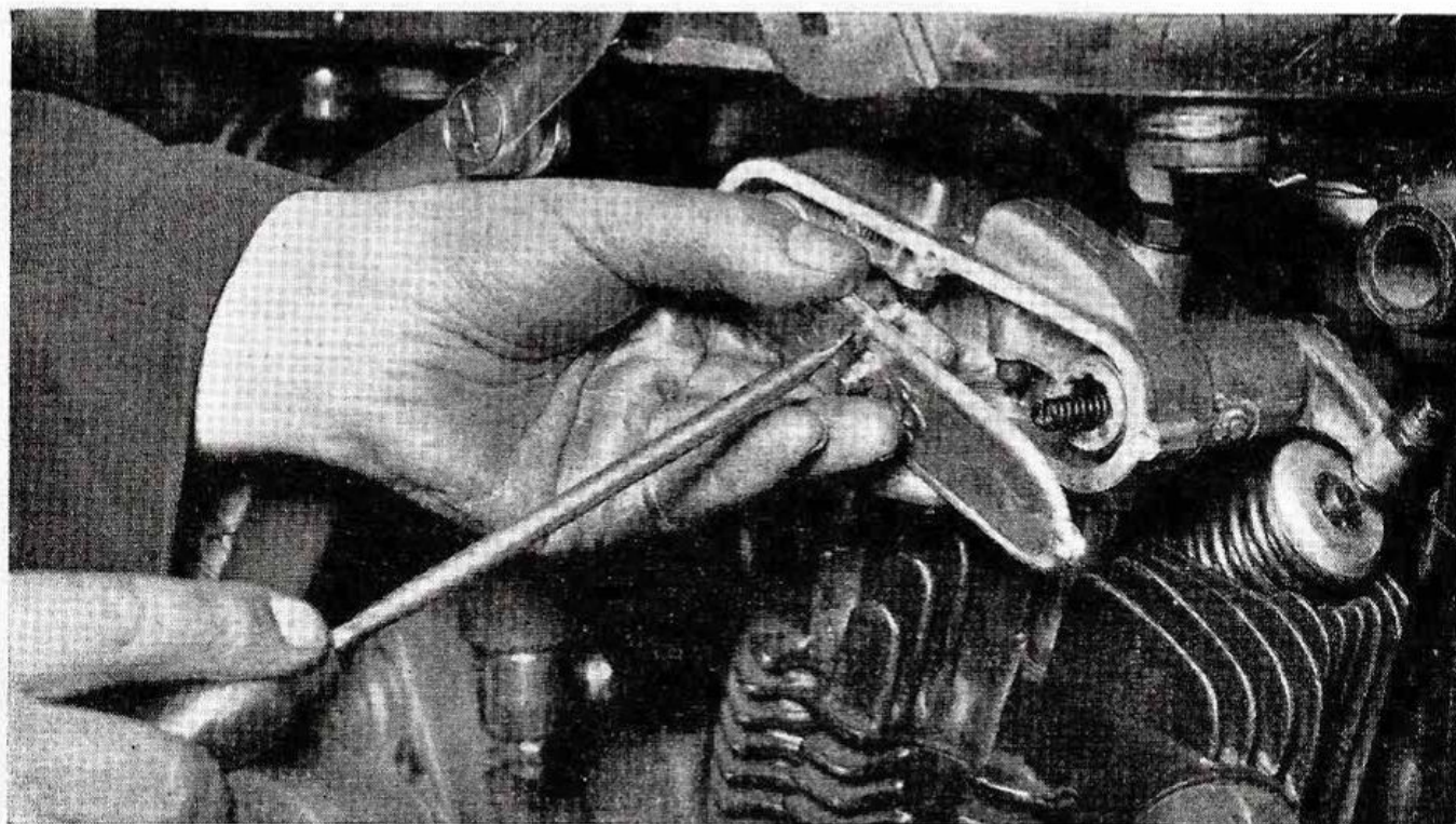
Fig. 1. —REMOVING ROCKER-BOX COVER.
