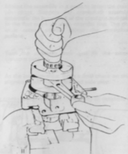
Fig. 24 Left crankcase held in vise using soft jaws to avoid damage.
