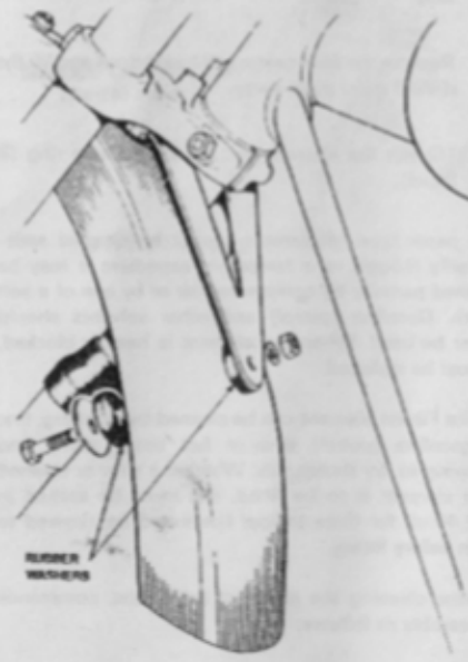
Fig. 64 Order of assembly of front fender fixings.
