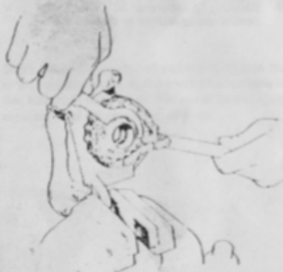
Fig. 42 Tapping lockwasher into castellations of countershaft sprocket locking.
