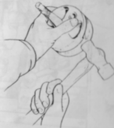
Fig. 20 Re-aligning crankcheeks using a soft faced hammer.
