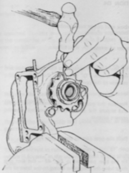
Fig. 43 Using a chain wrench to lock the countershaft sprocket.
