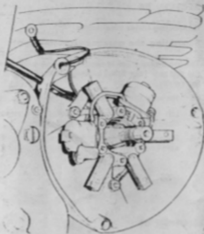
Fig. 10 Stator external connections.
