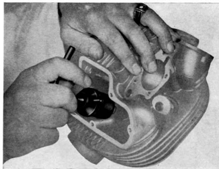
8 - Clamp for lapping the valve seats
