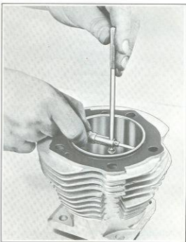
Figure 3C-4. Measuring Cylinder Bore
