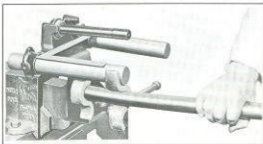
Figure 2F-15. Bending Bracket Legs Parallel
