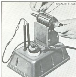
Figure 5E-4. Testing Armature for Short
