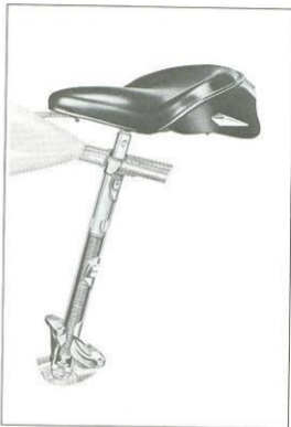
Figure 2H-1. Cutaway of Seat Post Springing
