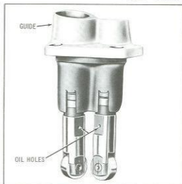
Figure 3D-3. Inserting Tappets on Guide
