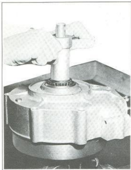
Figure 3E-17. Pressing Flywheel into Crankcase
