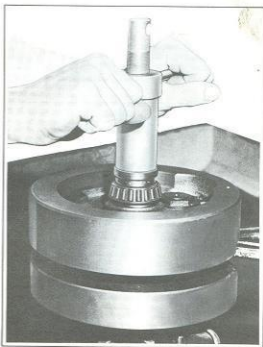
Figure 3E-16. Pressing Bearing on Sprocket Shaft
