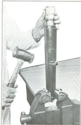
Figure 2F-17. Inserting New Oil Seal
