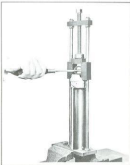
Figure 2F-19. Disassembling Shock Absorber (1966 & Earlier Shown)
