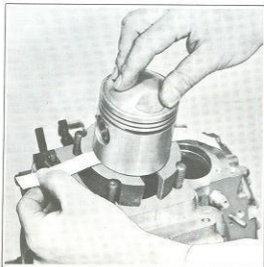
Figure 3C-11. Checking Rod Alignment
