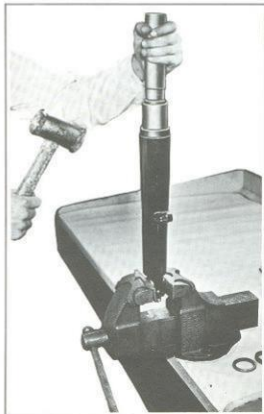
Figure 2F-7. Driving in Fork Slider Bushing
