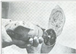
Figure 2J-12. Rough Sanding Outside Surface
