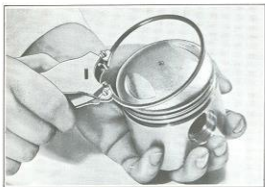
Figure 3C-9. Assembling Rings with Ring Expander
