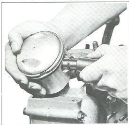
Figure 3C-14. Inserting Piston Pin Lock Ring
