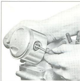
Figure 3C-2. Removing Piston Pin Lock Ring
