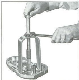
Figure 3D-6. Removing Pinion Shaft Cover Bushing
