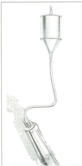
Figure 2F-2. Filling Hydraulic Fork with Oil
