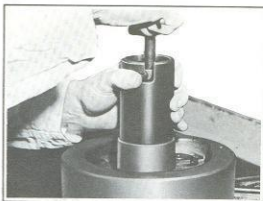
Figure 3E-7. Pulling Bearing from Sprocket Shaft
