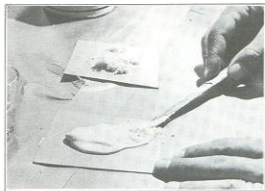
Figure 2J-2. Mixing Gel Coat and Glass Fibers
