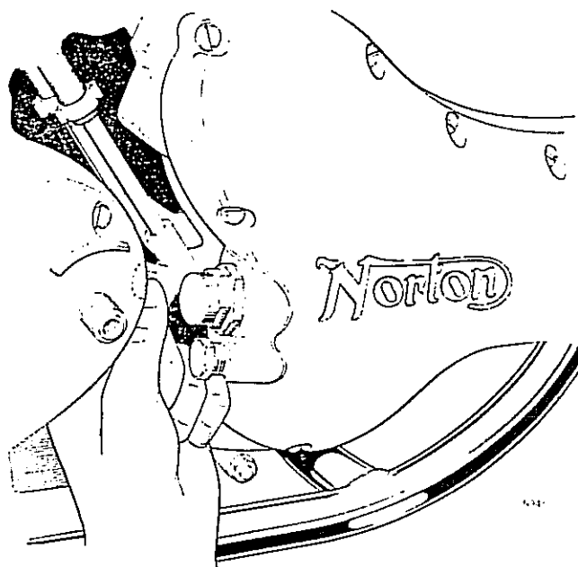
Fig. F1 Removing oil junction block securing bolt
