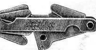
Fig. 12.—Setting the plug points
