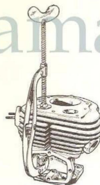
61-3340 Valve Spring Compressor Models C10, C11, M20, M21 (Use without adaptor)
